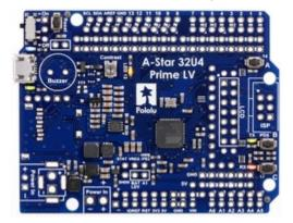
The A-Star 32U4 Prime LV can be powered from a 2.7 V to 11.8 V external source. The input voltage is regulated to 5 V by a TPS63061 switching step-up/step-down (buck-boost) converter from Texas Instruments. (We also make a standalone regulator [http://www.pololu.com/product/2123] based on this integrated circuit.)
