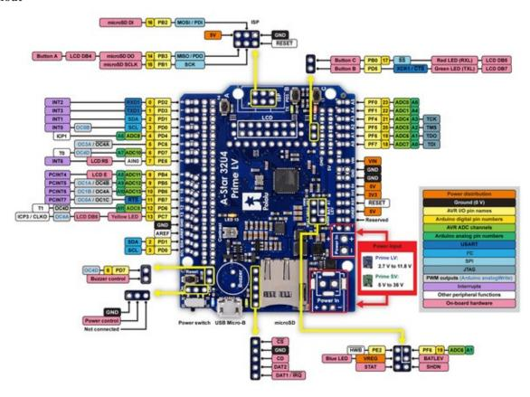
This diagram identifies the I/O and power pins on the A-Star 32U4 Prime (LV and SV versions); it is also available (along with the power distribution diagram below) as a **printable PDF** [http://www.pololu.com/file/download/a\_star\_32u4\_prime\_pinout\_power.pdf?file\_id=0J847] (1MB pdf). For more information about the ATmega32U4 microcontroller and its peripherals, see Atmel's ATmega32U4 documentation.
