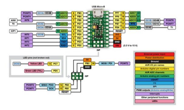
The diagram above identifies the I/O and power pins on the A-Star 32U4 Micro; it is also available as a **printable PDF** [http://www.pololu.com/file/download/a-star-32u4-micro-pinout.pdf?file\_id=0J796] (409k pdf). For more information about the ATmega32U4 microcontroller on this board, see **Atmel's ATmega32U4 documentation** [http://www.atmel.com/devices/atmega32u4.aspx].
