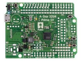
The A-Star 32U4 Prime SV can be powered from a 5 V to 36 V external source. The input voltage is regulated to 5 V by a 1 A ISL85410 switching step-down (buck) converter from Intersil. (We also make a **standalone regulator** [http://www.pololu.com/product/2831] based on this integrated circuit.)
