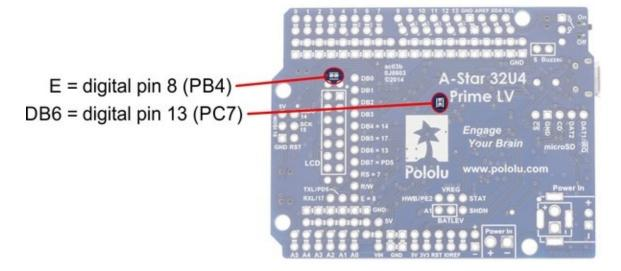
The AStar32U4PrimeLCD library provides functions to display data on a connected LCD. It is designed to gracefully handle alternate use of the LCD data lines by only changing pin states when needed for an LCD command, after which it will restore them to their previous states. This allows the LCD data lines to be used for other functions (such as pushbutton inputs and LED drivers).
