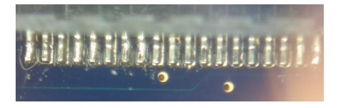
Turn the board and apply flux on the ground pins.
