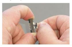
Place the connector onto the footprint on the evaluation board. Make sure that the guide tab beneath the connector fits into the guide hole in the PCB.
