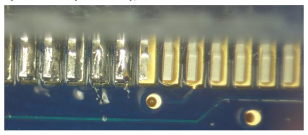
After soldering, you should make sure that there are no shorts circuits between pins.
