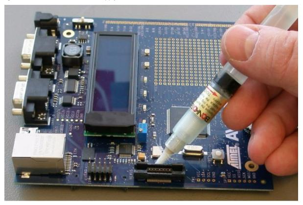
Make sure that the connector is firmly seated on the footprint, and start by soldering the corners.
