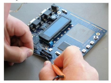
When all corners are soldered, check that connector is still firmly seated. It is still possible to push the connector down and re-heat corner pins if you need to adjust a bit.
