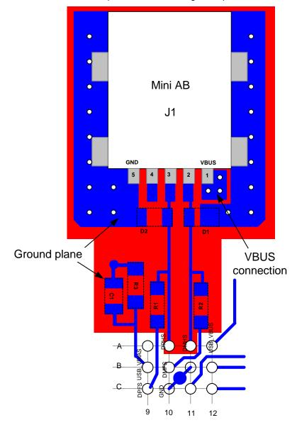
Figure 3-2. Standard Mini AB Receptacle - USB Routing Example with BGA144 Package
