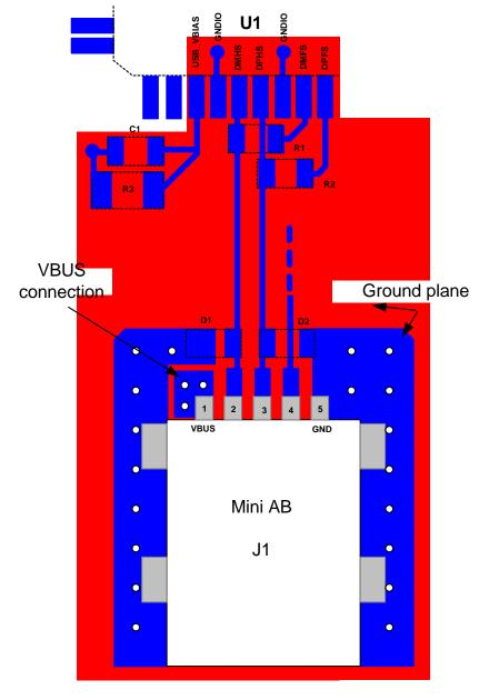
Figure 3-1. Standard Mini AB Receptacle - USB Routing Example with QFP144 Package
