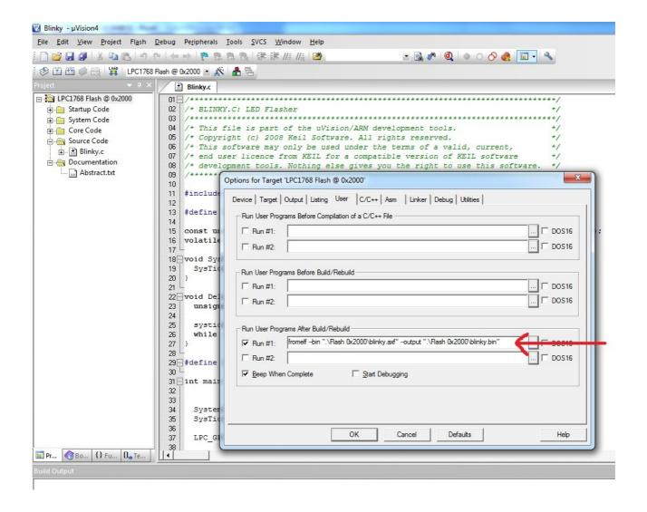
Insert the user command in Run #1 ticking the check box. After compile and build the entire project, from elf it creates hex file along with the hex file there will be another file with the extension .axf. This user command is used to convert .axf file to .bin. Here in fig. Above blinky.axf is converted to blinky.bin which is used for drag drop programming with the USB boot-loader that allows you to enumerate the board as a Mass Storage Device.
