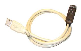
Before the cable can be used on a given computer, it must be identified to the Adept software by adding its serial number or alphanumeric ID string to the device table in the Adept software. Every cable is given a unique serial number and default "DCabUsb" ID string. The USB administrator tool in the Adept software can automatically identify a newly attached cable and add it to the device table. Once the cable ID is in the device table, it can be used to configure Xilinx devices.
