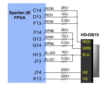
Figure 13. VGA pin definitions and Basys2 circuit
