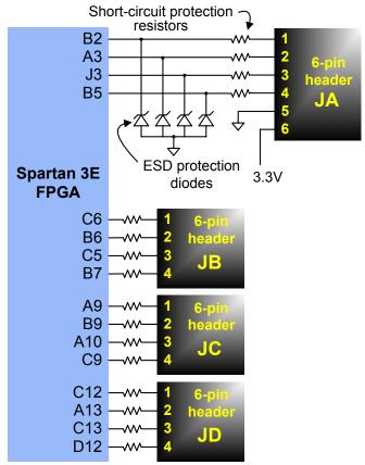
Figure 18. Basys2 Pmod connector circuits
