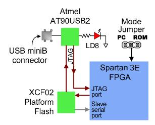
Figure 4. Basys2 Programming Circuits
