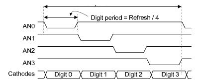
Figure 8. Multiplexed 7seg display timing
