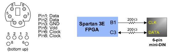
Figure 9. PS/2 connector and Basys2 PS/2 circuit
