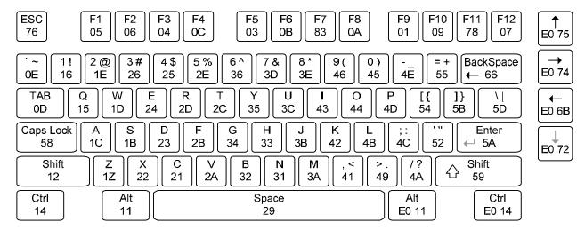
Figure 11. Keyboard scan codes
