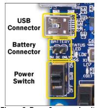
Figure 2. Basys2 power circuits
