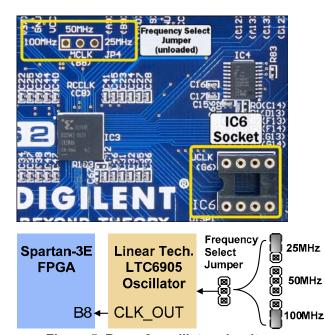
Figure 5. Basys2 oscillator circuits
