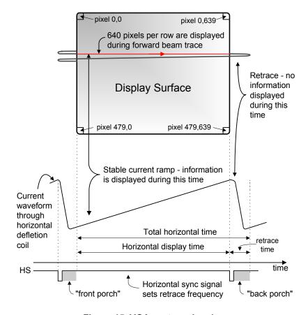
Figure 15. VGA system signals
