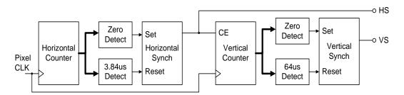
Figure 15. VGA display controller block diagram.
