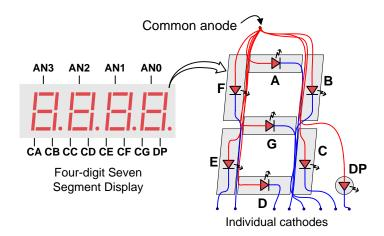
Figure 18. Common anode circuit node.
