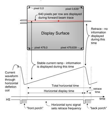
Figure 13. VGA horizontal synchronization.
