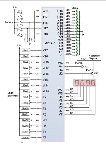
Figure 16. General purpose I/O devices on the Basys3.
