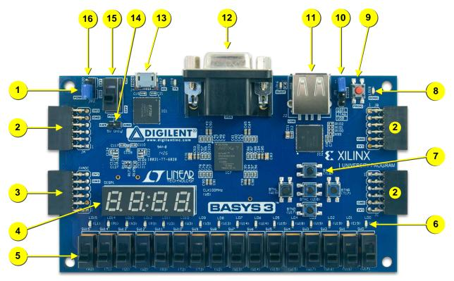
Figure 1. Basys3 FPGA board with callouts.
