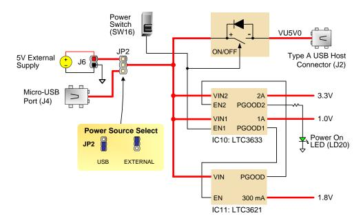
Figure 2. Basys3 power circuit.
