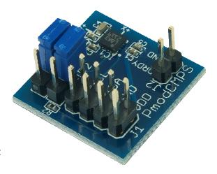
There are two eight bit registers for each axis. Once one data register is read, the other five data registers must be read before any new data can be written to those registers.
