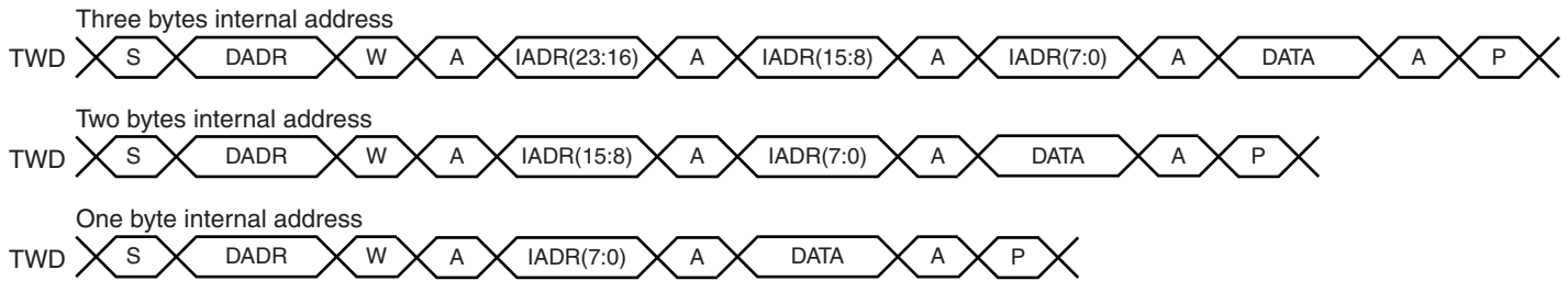
Figure 31-11. Master Write with One, Two or Three Bytes Internal Address and One Data Byte
