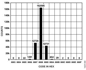
Figure 14. Histogram of a DC Input at the Code Center,  $V_{REF} = 5 V$
