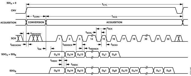
Figure 39. Chain Mode Serial Interface Timing
