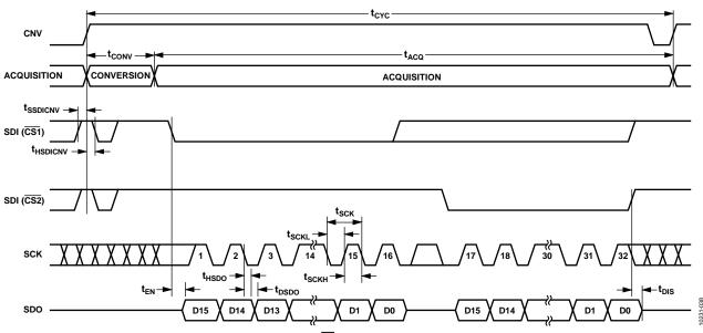
Figure 37. 4-Wire CS Mode Serial Interface Timing
