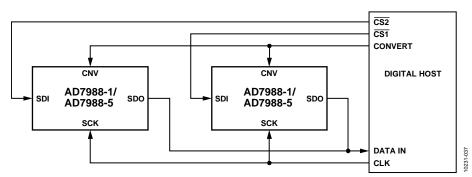
Figure 36. 4-Wire  $\overline{CS}$  Mode Connection Diagram
