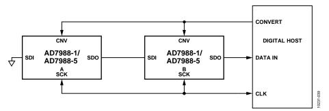
Figure 38. Chain Mode Connection Diagram
