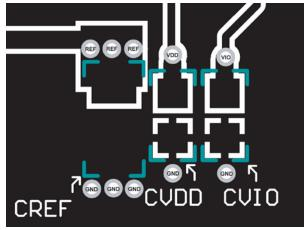
Figure 43. Example Layout of the AD7988-x (Bottom Layer)
