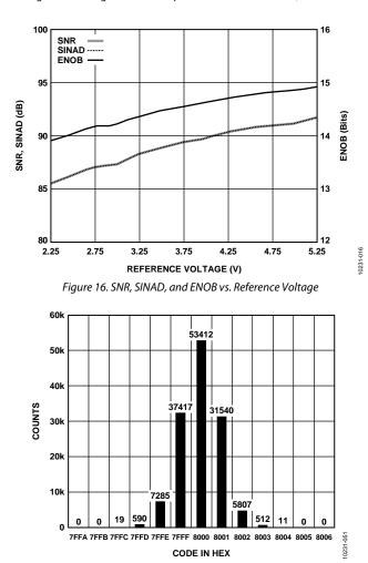
Figure 17. Histogram of a DC Input at the Code Center,  $V_{REF} = 2.5 V$
