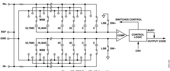
Figure 29. ADC Simplified Schematic
