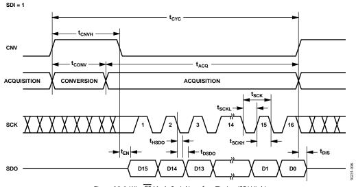
Figure 35. 3-Wire CS Mode Serial Interface Timing (SDI High)
