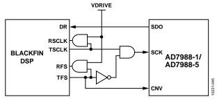
Figure 41. Evaluation Board Connection to Blackfin Sport Interface
