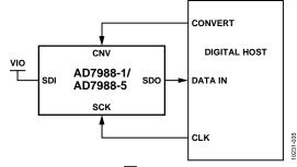
Figure 34. 3-Wire CS Mode Connection Diagram
