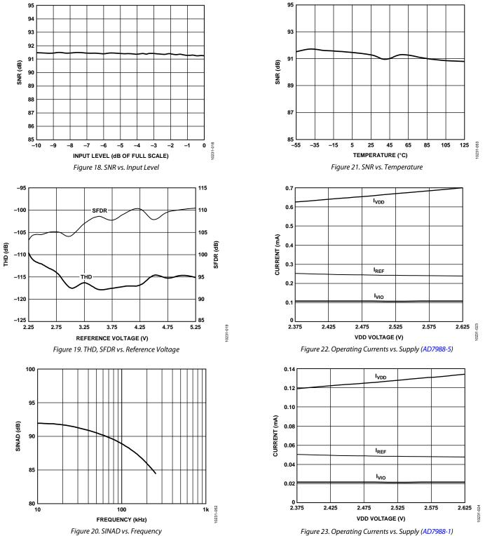
Figure 23. Operating Currents vs. Supply (AD7988-1)
