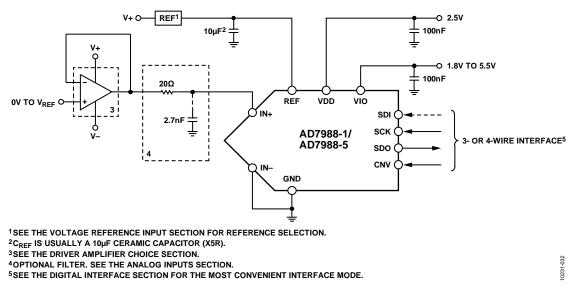
Figure 31. Typical Application Diagram with Multiple Supplies
