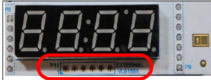
Figure 27. Connections for external VL6180X
