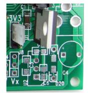
Fig. 7: Image showing header J7 with translucent jumper in place. J7 is located just above J8 (J7 legend is obscured in this image)
