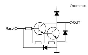
Fig. 15: Circuit diagram of each open collector driver.
