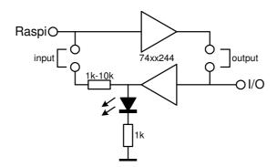
Fig. 8: The circuit diagram for I/O ports 4-12
