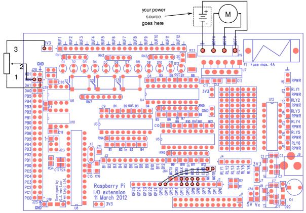
Fig. 30: Wiring diagram for the combined potmot test.
