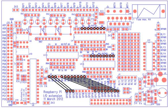
Fig. 31: Wiring diagram for the decoder test.
