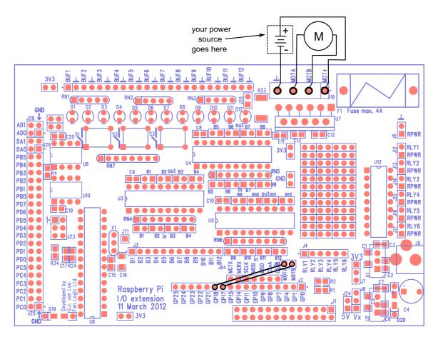
Fig. 20: The wiring diagram for the test program motor.
