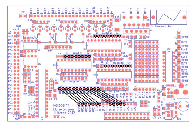
Fig. 13: The wiring diagram necessary to run the Gertboard LED test program, leds
