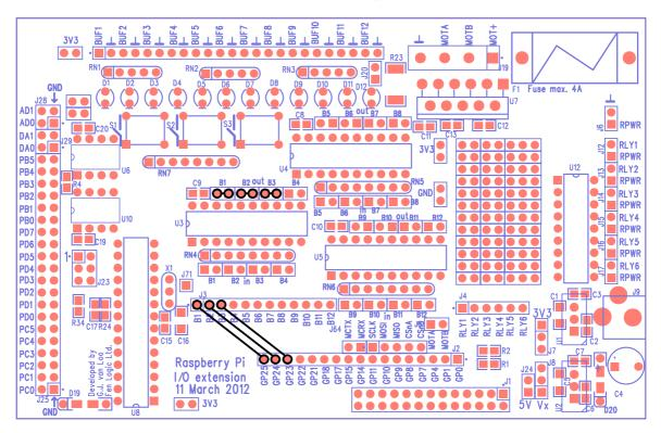
Fig. 12: This type of diagram is much more effective at showing how straps connect pins together on the board, so from now onwards, we will use these type of diagrams to show wiring arrangements.
