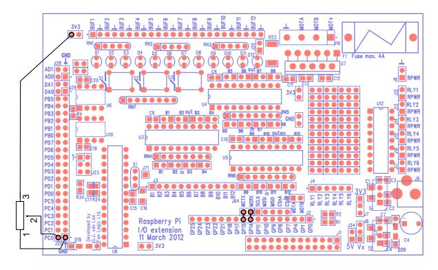
Fig. 29: Wiring diagram for the sketch AnalogInSerial/AnalogReadSerial.
