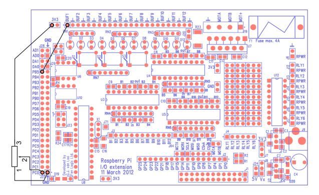
Fig. 28: Wiring diagram for the AnalogInput sketch.
