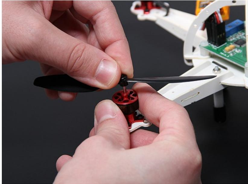
Be sure to install propellers in the correct rotation direction (see photo below for reference):
