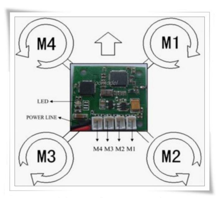
The power cables (line) on this, is on a different place, but the motor config. is the same
