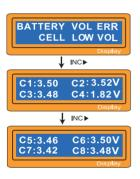
The processor found that the voltage of one of the cell in the Lithium battery pack is too low.
