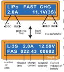
You can set up the charging current and the voltage of the battery pack being charged. As you press Start/Enter button the voltage confirmation will be displayed. And then, if you confirm the voltage and current, press Start/Enter button again to start charging.
