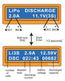
The value of discharge current on the left side of screen may not exceed 1C for a maximum safety and the final voltage on the right should not be under the voltage level that is recommended by the battery manufacturer to avoid deep discharging. To start to discharge, press Start/Enter key for more than 3 seconds.
