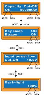
This program sets the maximum charge capacity that will be supplied to the battery during charge. If the delta-pack voltage is not detected nor the safety timer expired by any reason, this feature will automatically stop the process at the selected capacity value.
