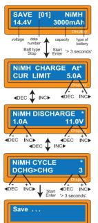
with the battery type you set up. The example shows the battery pack of NiMH, 12cells and 3000mAh of capacity.
