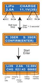
After setting the current and voltage press Start/Enter key for more than 3 seconds to start the process.
