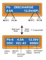
Set discharge current on the left and final voltage on the right. The discharge current ranges from 0.1 to 5.0A.
