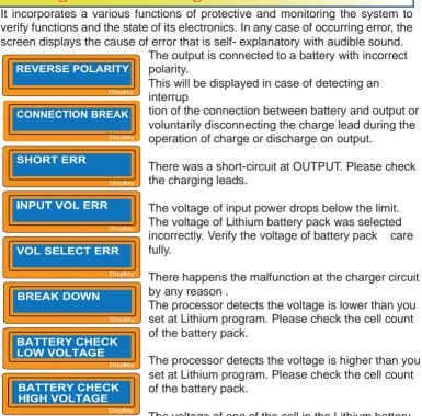
The processor detects the voltage is higher than you set at Lithium program. Please check the cell count
