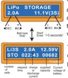
You can set up the current and the voltage of the battery pack to be charged. The current will be used for charge or discharge the battery to reach the 'storage' level of voltage.
