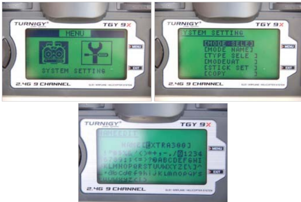
Menu "MODE NAME" allows you to assign a name to each of the 8 model memories.
