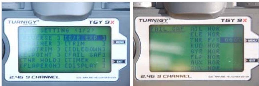
The failsafe function to define what behavior the receiver should adopt towards the servos.
