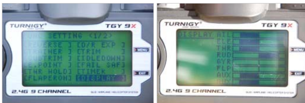
The sub menu "DISPLAY" achieves a kind of 'photograph' of the adjustment status.
