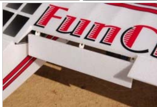
AIR BRAKES function enables the aerodynamic braking on an airplane, lower or control its flight speed or increase its lift.
