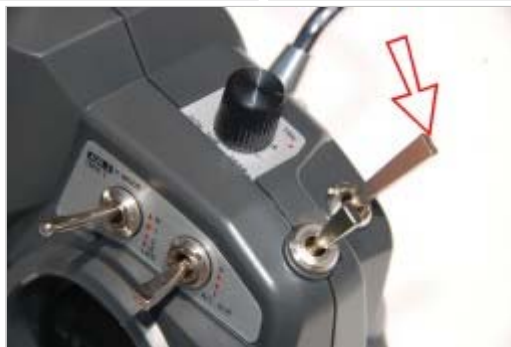
The TGY 9x has only one timer that can start and stop at will with the international (top right rear).
