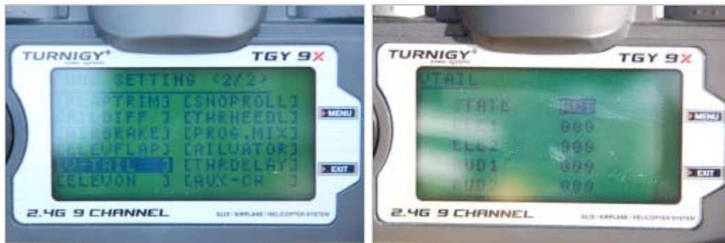
VTAIL function allows mixing depth and direction on models whose tail is in V.
