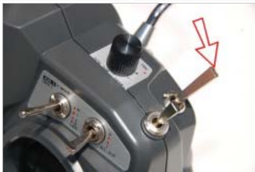
The submenu "REVERSE" is very useful, it can change the direction of operation of each servo to fit the model ..
