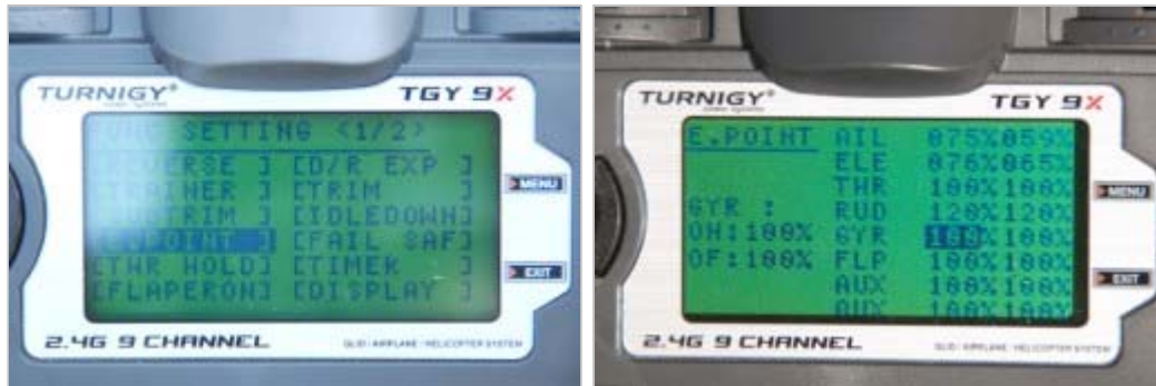
END POINT function adjusts for each channel, the maximum deflection.
