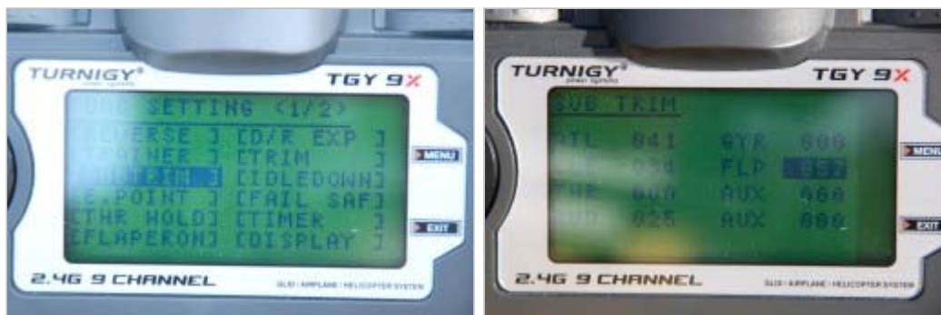
SUB TRIM function can precisely adjust the neutral position of the servo arm.
