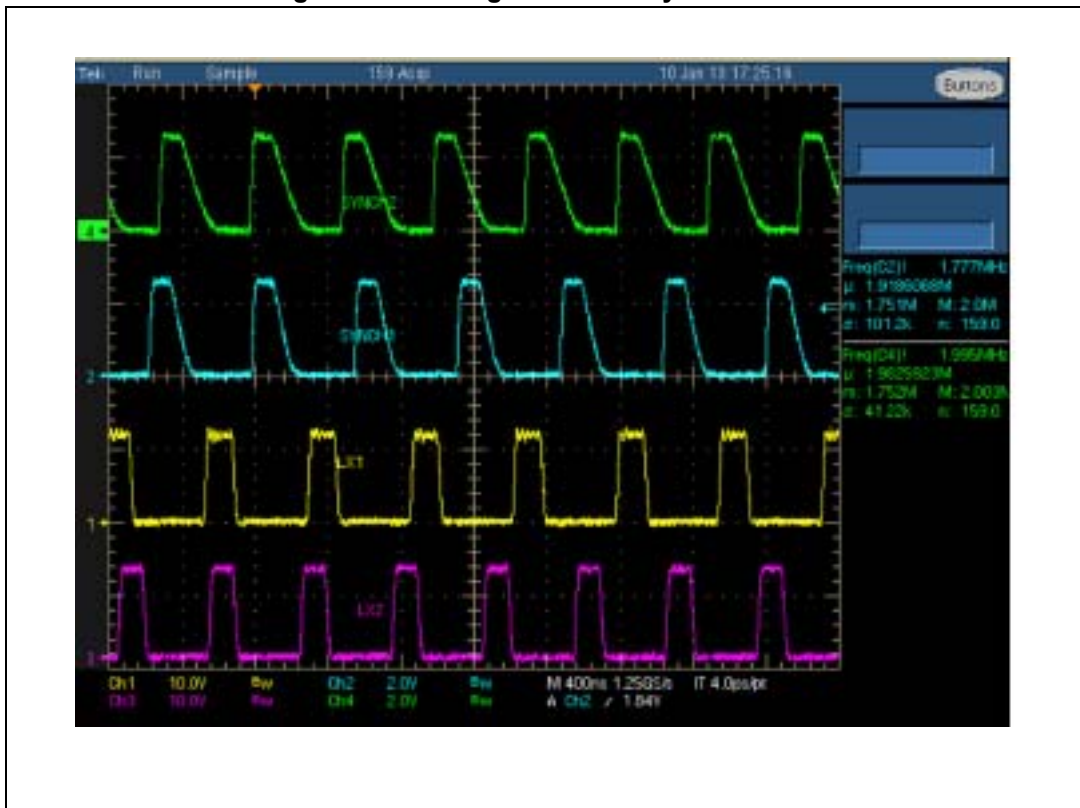
Figure 28. Two regulators not synchronized
