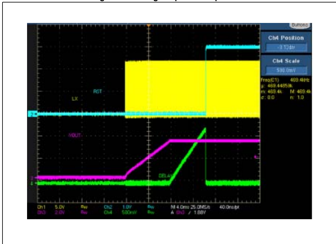
Figure 27. Voltage supervisor operation
