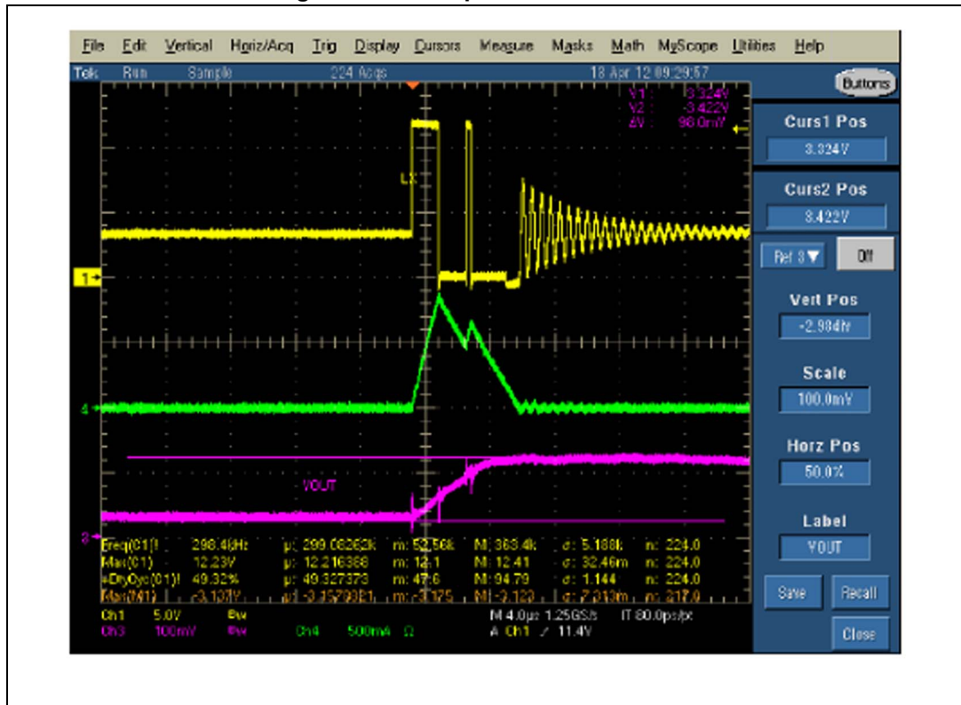
Figure 11. LCM operation at zero load
