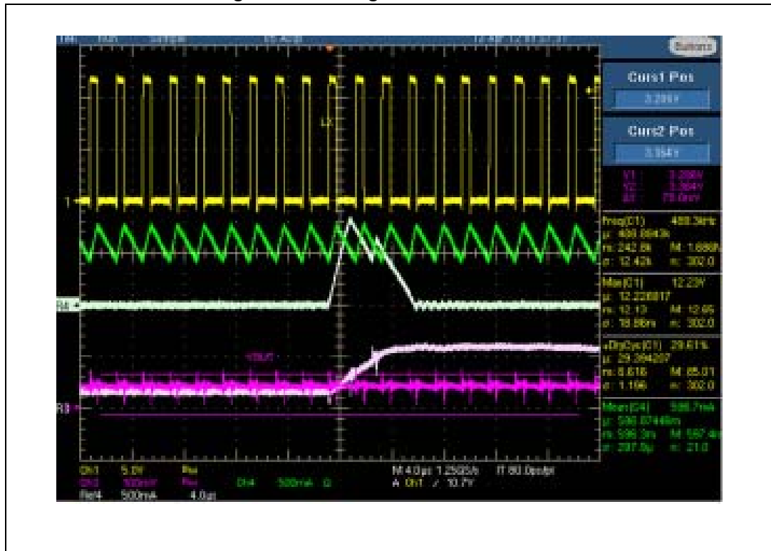
Figure 14. The regulator works in CCM
