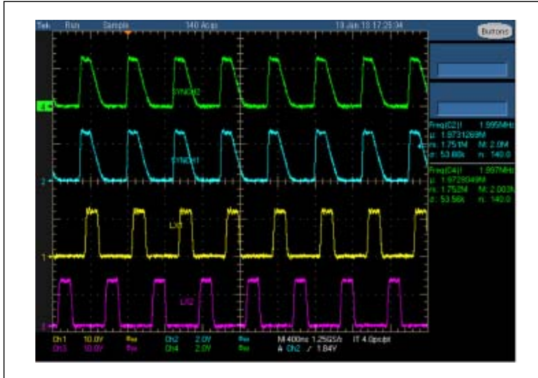
Figure 29. Two regulators synchronized
