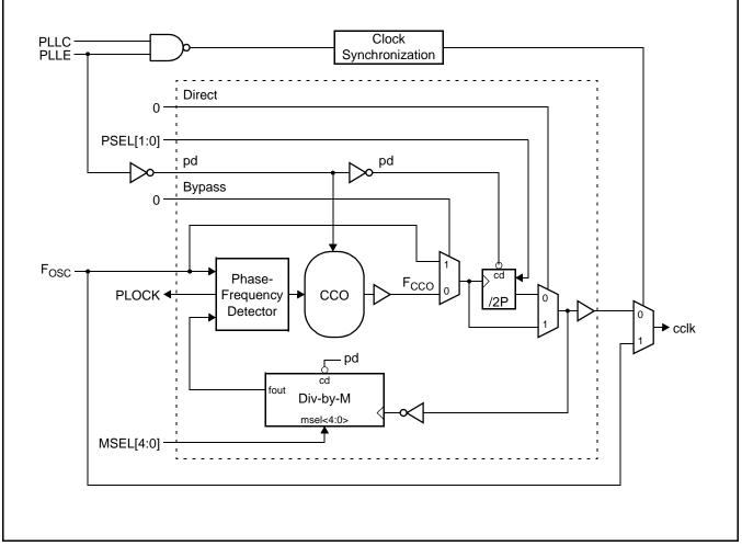
Figure 15: PLL Block Diagram
