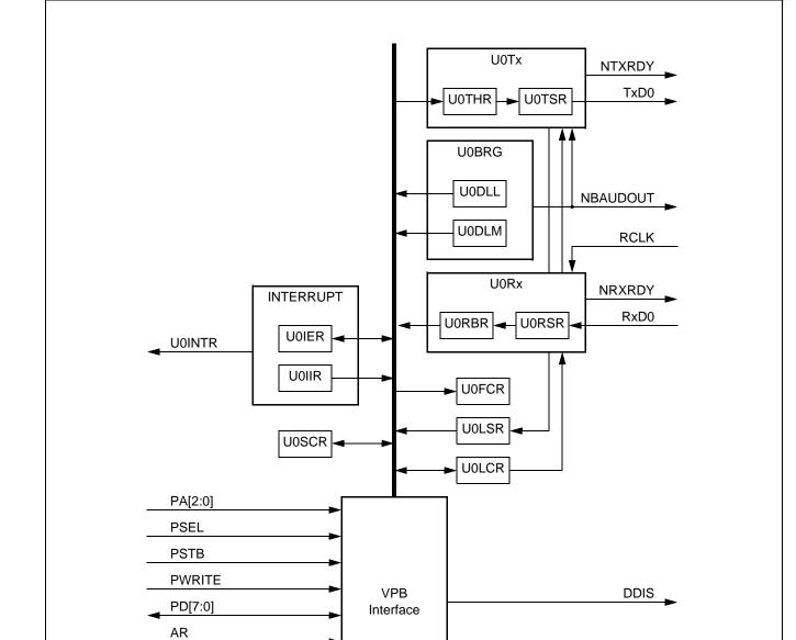
Figure 22: UART0 Block Diagram
