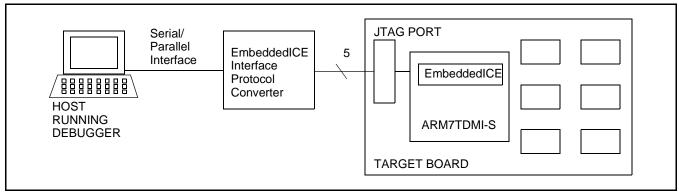
Figure 51: EmbeddedICE Debug Environment Block Diagram
