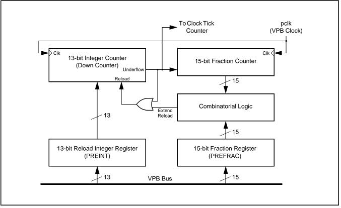
Figure 45: RTC Prescaler block diagram
