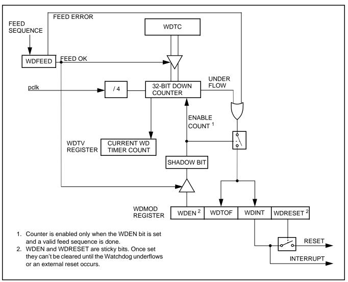
Figure 46: Watchdog Block Diagram
