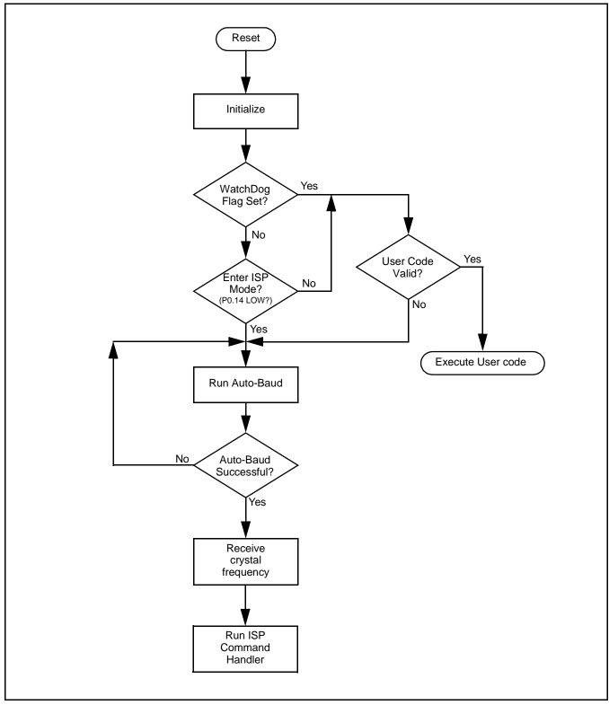
Figure 48: Boot Process flowchart (Bootloader revisions before 1.61)
