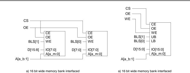
a) 16 bit wide memory bank interfaced to 16 bit memory chips
