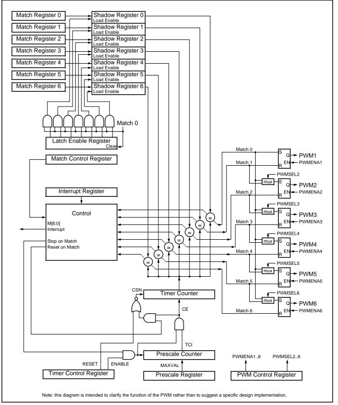
Figure 42: PWM block diagram
