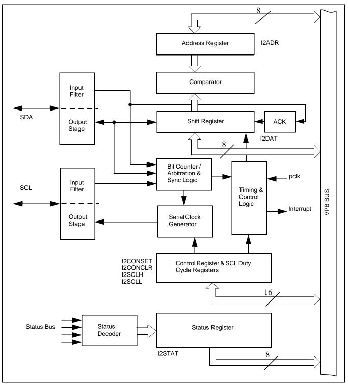
Figure 32: I<sup>2</sup>C Architecture
