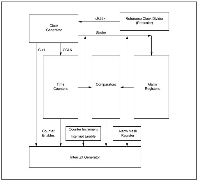
Figure 44: RTC block diagram
