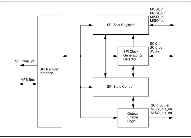
Figure 34: SPI Block Diagram
