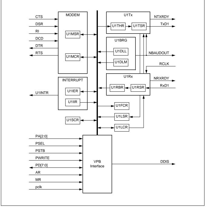
Figure 23: UART1 Block Diagram
