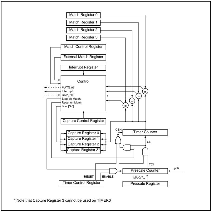
Figure 41: Timer block diagram
