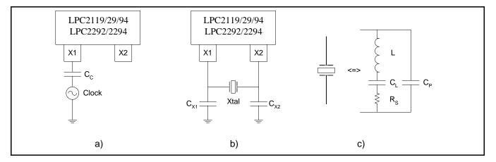
Figure 12: Oscillator modes and models: a) *slave mode* of operation, b) *oscillation mode* of operation, c) external crystal model used for C<sub>X1/X2</sub> evaluation
