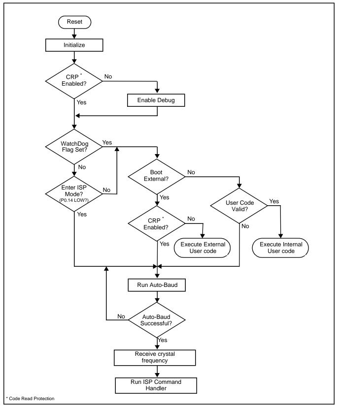
Figure 49: Boot Process flowchart (Bootloader revisions 1.61 and later)
