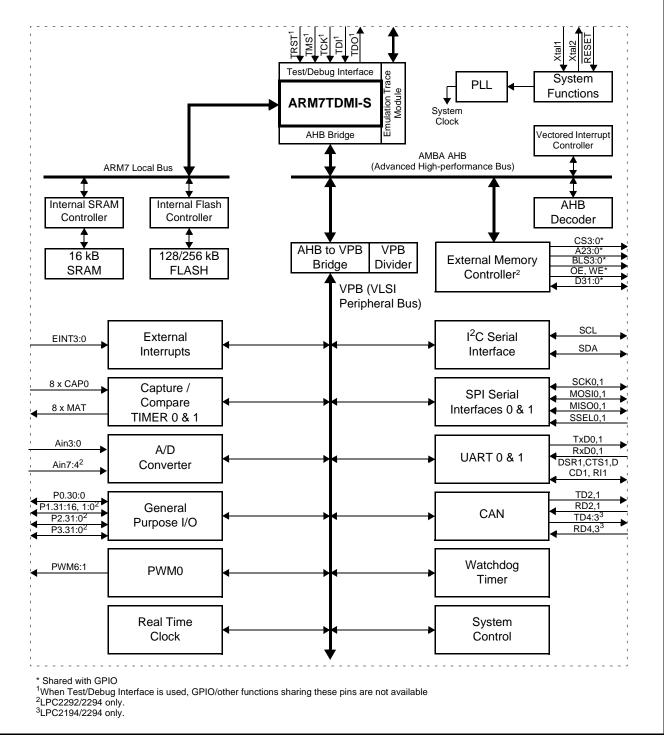
Figure 1: LPC2119/2129/2194/2292/2294 Block Diagram
