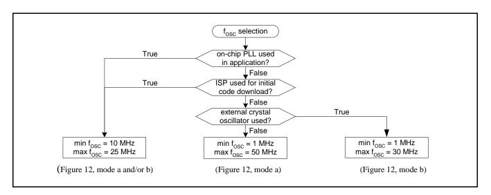
Figure 13: F<sub>OSC</sub> selection algorithm
