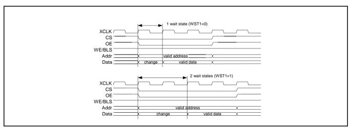
Figure 10: External memory read access (WST1=0 and WST1=1 examples)
