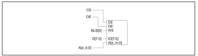
Figure 9: 8 Bit Bank External Memory Interface
