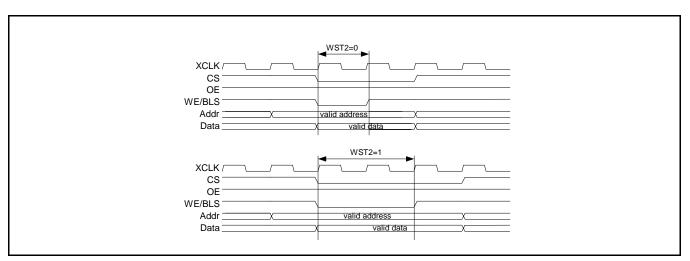
Figure 11: External memory write access (WST2=0 and WST2=1 examples)
