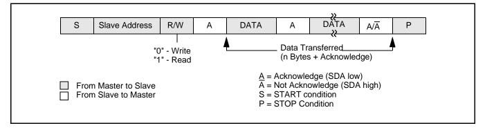
Figure 26: Format in the master transmitter mode
