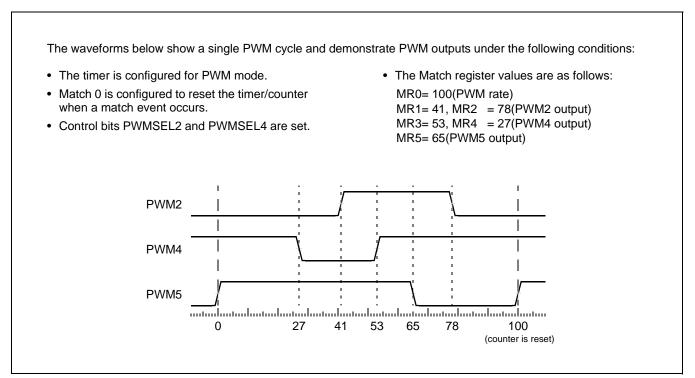
Figure 43: Sample PWM waveforms
