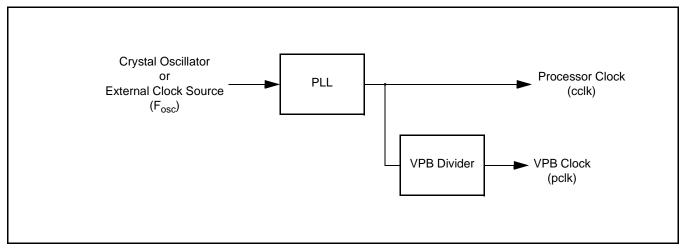
Figure 17: VPB Divider Connections
