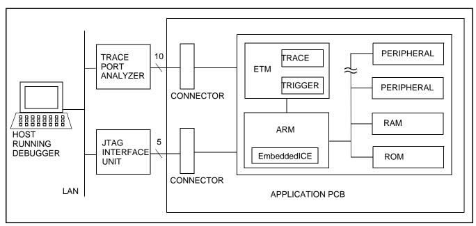
Figure 52: ETM Debug Environment Block Diagram
