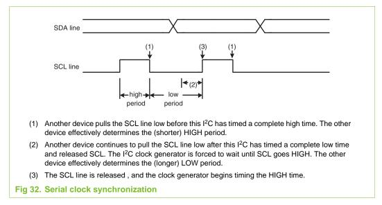
A slave may stretch the space duration to slow down the bus master. The space duration may also be stretched for handshaking purposes. This can be done after each bit or after a complete byte transfer. the I<sup>2</sup>C block will stretch the SCL space duration after a byte has been transmitted or received and the acknowledge bit has been transferred. The serial interrupt flag (SI) is set, and the stretching continues until the serial interrupt flag is cleared.
