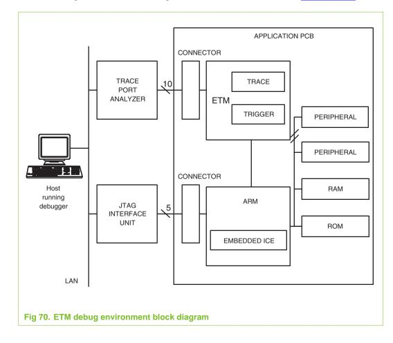
The block diagram of the ETM debug environment is shown below in Figure 23–70.
