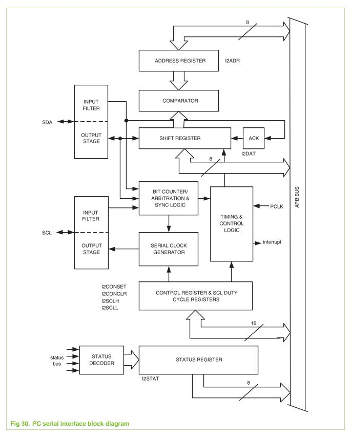
The output for I<sup>2</sup>C is a special pad designed to conform to the I<sup>2</sup>C specification.
