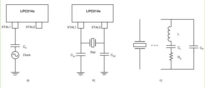
Fig 7. Oscillator modes and models: a) slave mode of operation, b) oscillation mode of operation, c) external crystal model used for  $C_{X1}/_{X2}$  evaluation
