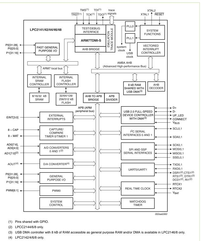
Fig 1. LPC2141/2/4/6/8 block diagram
