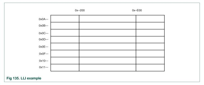
The first LLI, stored at 0x20000, defines the first block of data to be transferred, which is the data stored between addresses 0x0A200 and 0x0AE00:
