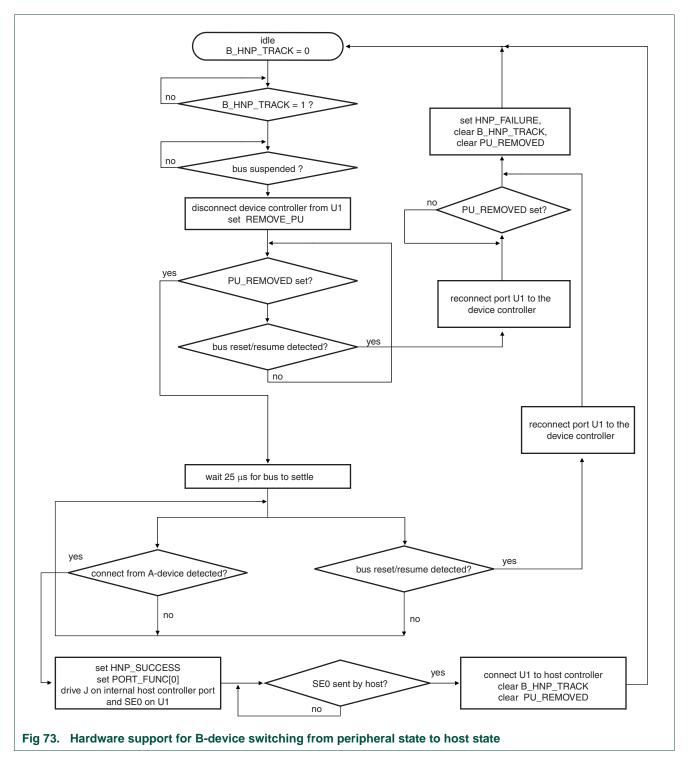
Figure 15–74 shows the actions that the OTG software stack should take in response to the hardware actions setting REMOVE\_PU, HNP\_SUCCESS, AND HNP\_FAILURE. The relationship of the software actions to the Dual-Role B-Device states is also shown. B-device states are in bold font with a circle around them.
