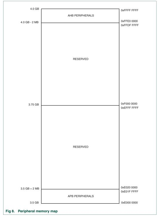
Figure <u>9</u> and <u>Table 2–9</u> show different views of the peripheral address space. Both the AHB and APB peripheral areas are 2 megabyte spaces which are divided up into 128 peripherals. Each peripheral space is 16 kilobytes in size. This allows simplifying the address decoding for each peripheral.
