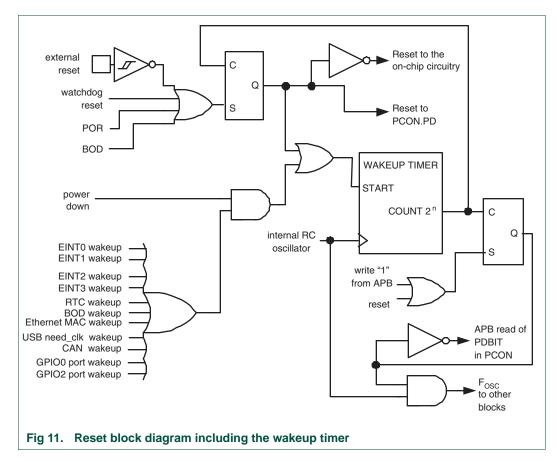
On the assertion of any of reset sources (POR, BOD reset, External reset and Watchdog reset), the IRC starts up. After the IRC-start-up time (maximum of 60  $\mu$ s on power-up) and after the IRC provides stable clock output, the reset signal is latched and synchronized on the IRC clock. Then the following two sequences start simultaneously :
