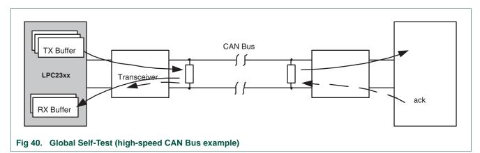
Initiating a Global Self-Test is similar to a normal CAN transmission. In this case the transmission of a CAN message(s) is initiated by setting Self Reception Request bit (SRR) in conjunction with the selected Message Buffer bits (STB3, STB2, STB1) in the CAN Controller Command register (CANCMR).
