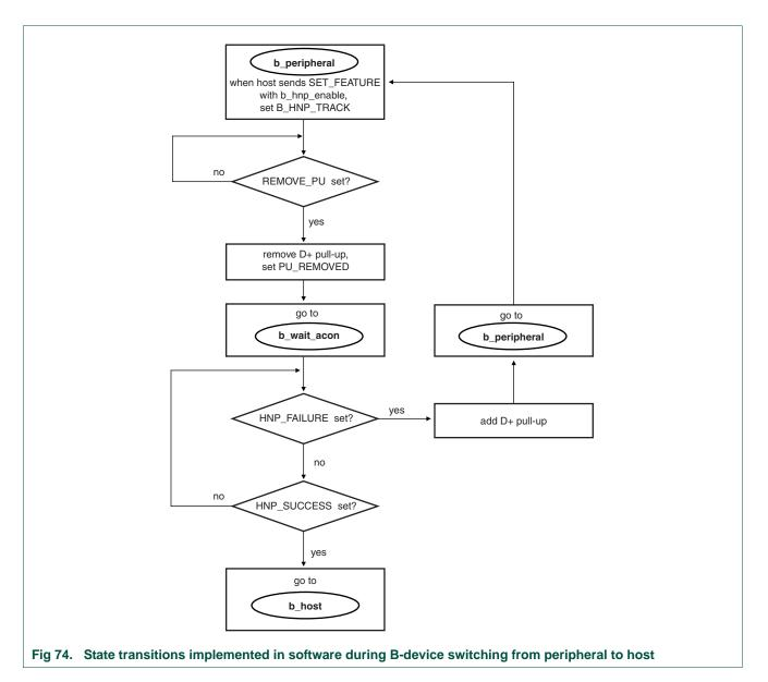
Note that only the subset of B-device HNP states and state transitions supported by hardware are shown. Software is responsible for implementing all of the HNP states.
