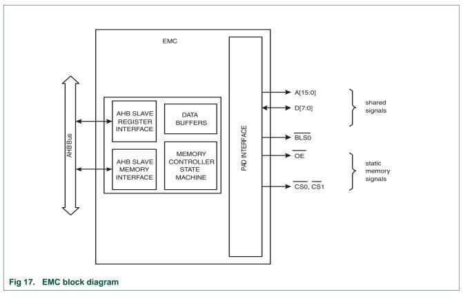
Figure 5–17 shows a block diagram of the EMC.
