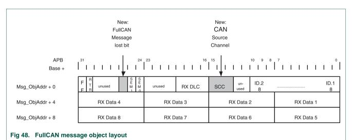
The new message lost bit (MsgLst) is introduced to indicate whether more than one FullCAN message has been received since last time this message object was read. For more information the CAN Source Channel (SCC) of the received FullCAN message is added to Message Object.
