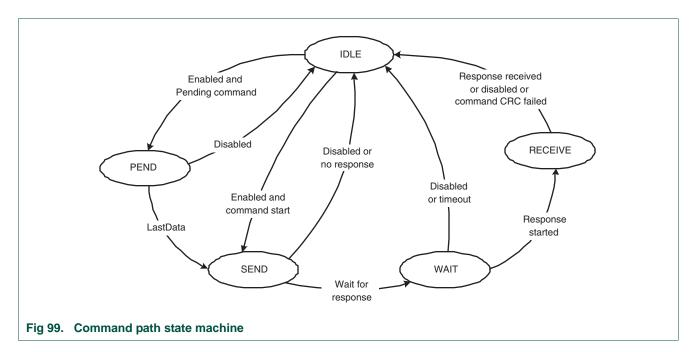
When the WAIT state is entered, the command timer starts running. If the timeout<sup>1</sup> is reached before the CPSM moves to the RECEIVE state, the timeout flag is set and the IDLE<sup>2</sup> state is entered.
