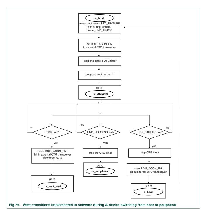
Note that only the subset of A-device HNP states and state transitions supported by hardware are shown. Software is responsible for implementing all of the HNP states.
