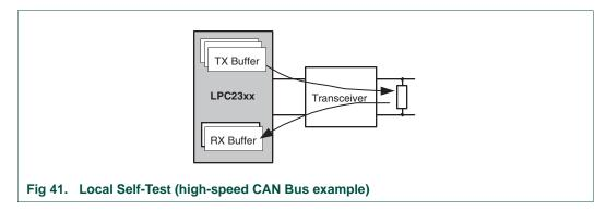
A message transmission is initiated by setting Self Reception Request bit (SRR) in conjunction with the selected Message Buffer(s) (STB3, STB2, STB1).
