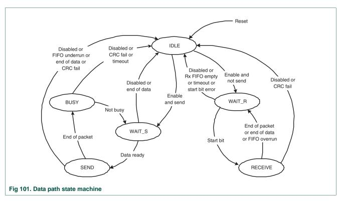
• IDLE: The data path is inactive, and the MCIDAT[3:0] outputs are in HI-Z. When the data control register is written and the enable bit is set, the DPSM loads the data counter with a new value and, depending on the data direction bit, moves to either the WAIT\_S or WAIT\_R state.
