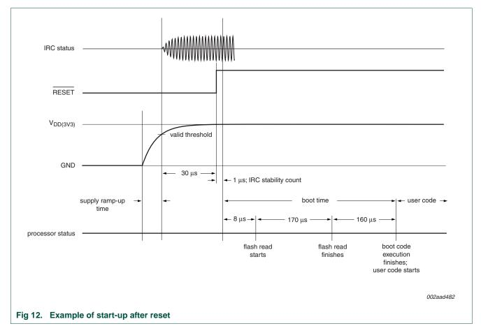
The various Resets have some small differences. For example, a Power On Reset causes the value of certain pins to be latched to configure the part.
