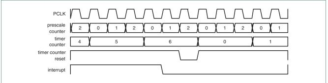
Fig 121. A timer cycle in which PR=2, MRx=6, and both interrupt and reset on match are enabled.
