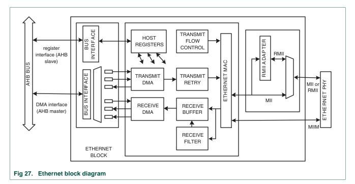
Figure 11–27 shows the internal architecture of the Ethernet block.
