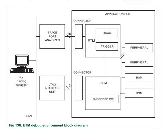
The block diagram of the ETM debug environment is shown below in Figure 31–136.
