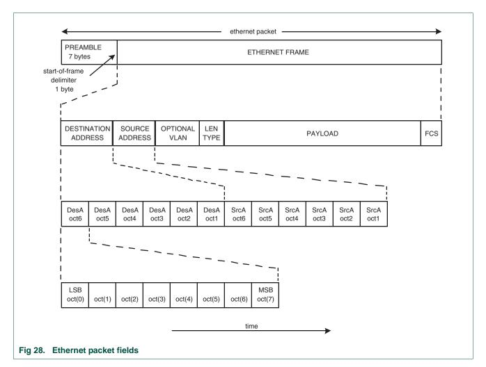
A packet consists of a preamble, a start-of-frame delimiter and an Ethernet frame.
