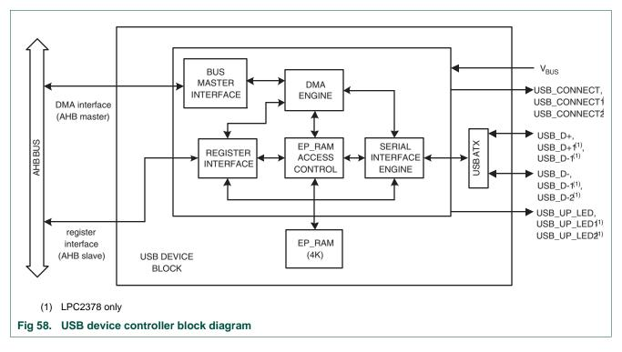
The architecture of the USB device controller is shown below in Figure 13–58.
