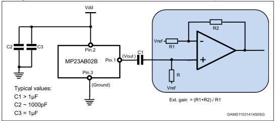
Figure 3. MP23AB02B electrical connections and external component values
