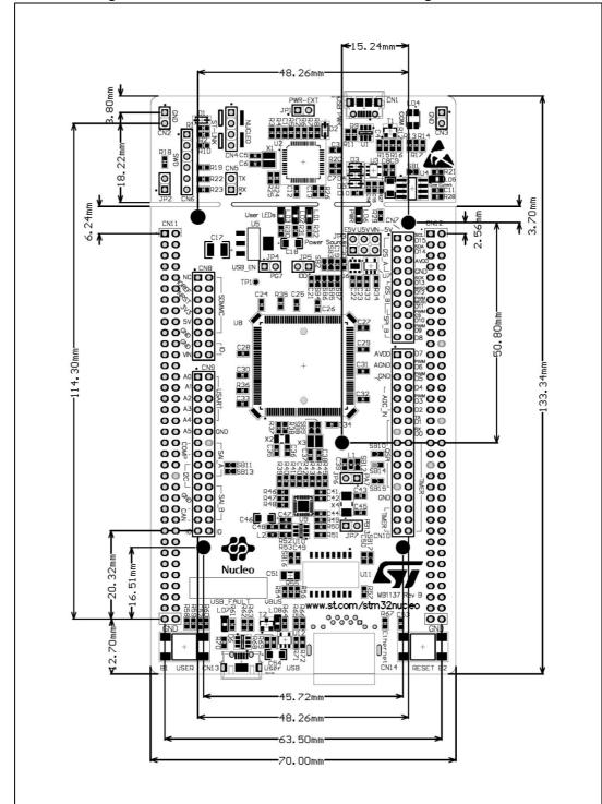
Figure 18. Nucleo-144 board mechanical drawing in millimeter
