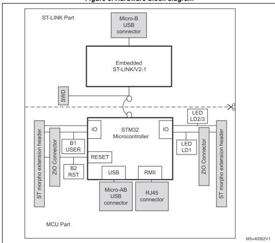
Figure 3. Hardware block diagram
