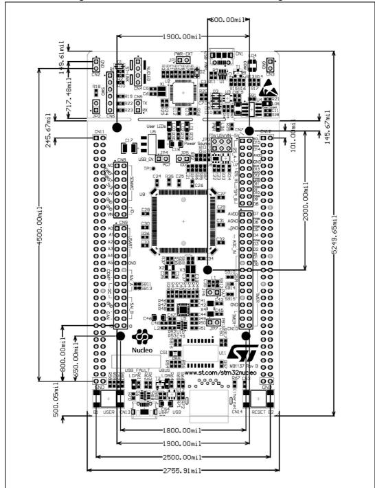
Figure 19. Nucleo-144 board mechanical drawing in mil
