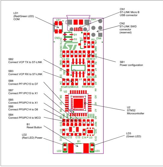
Figure 3. Top layout view of the Nucleo-32 board
