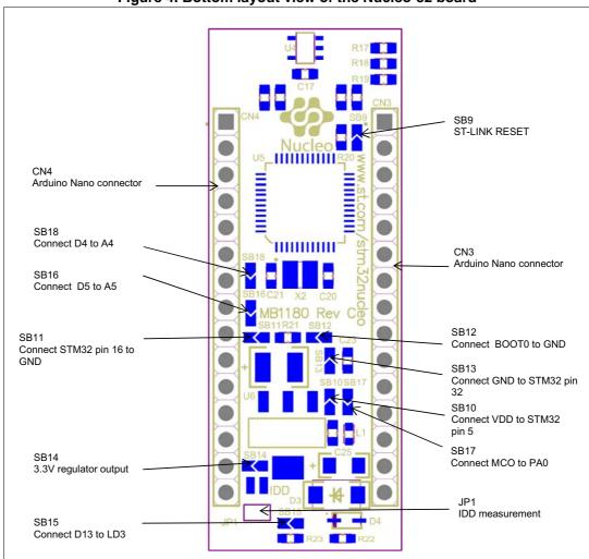
Figure 4. Bottom layout view of the Nucleo-32 board
