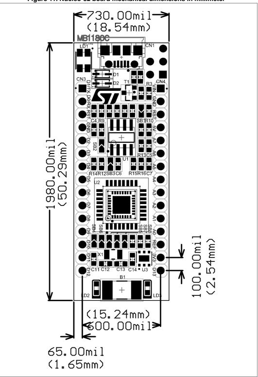
Figure 11. Nucleo-32 board mechanical dimensions in millimeter
