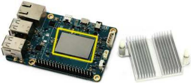
3. There is another thermal interface material on the heatsink. Please remove the film on it when you use this part.
