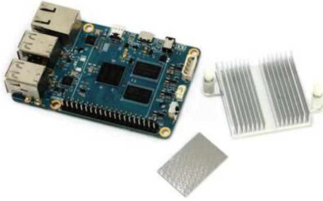
2. Place the thermal interface material on CPU and Memory.
