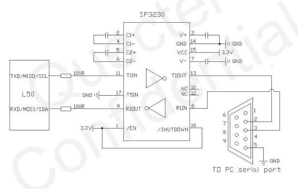
Figure 10: RS-232 level shift circuit
