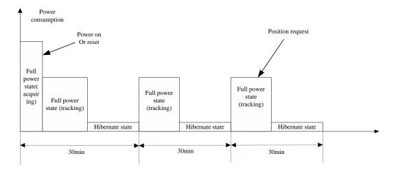
Figure 3: PTF timing sequence
