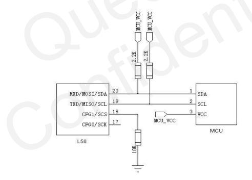
Figure 12: I2C design reference for L50 module
