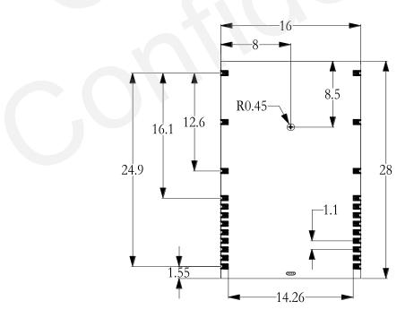
Figure 17: L50 Bottom view (Unit:mm)
