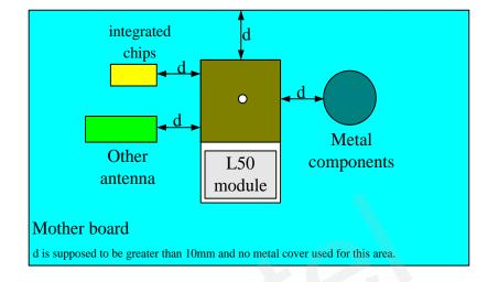
Figure 15: L50 module placement guide
