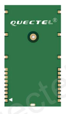
Figure 20: Bottom view of module
