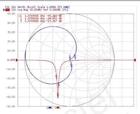
Figure 14: Patch antenna test result with ground plane 29.5mm×28.5mm
