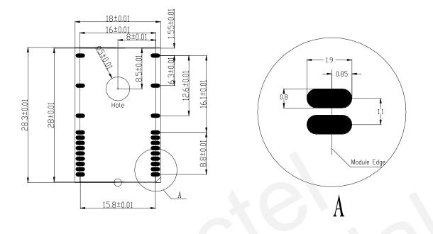
Figure 18: Recommended footprint (Unit:mm)
