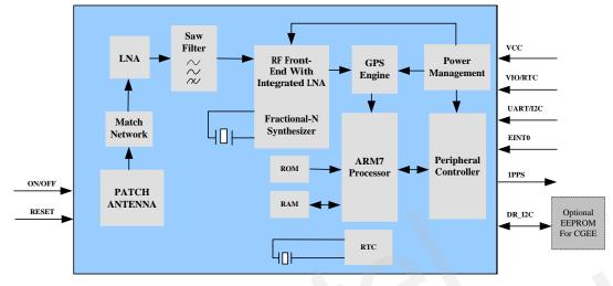
Figure 1: Functional diagram for L50
