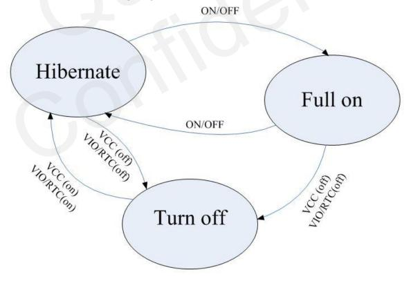
**Figure 8: State conversion of module**
