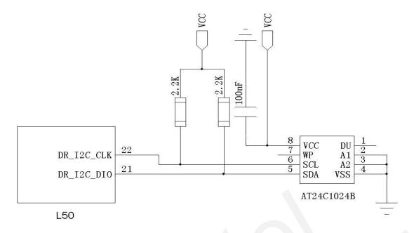
Figure 13: Reference design for CGEE function
