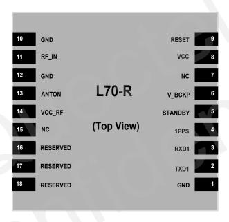
Figure 2: Pin Assignment
