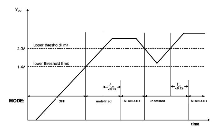
The threshold limit where the device switches from OFF to STAND-BY mode is between  $V_{\rm DD}$  =1.4V and  $V_{\rm DD}$  =2.0V.
