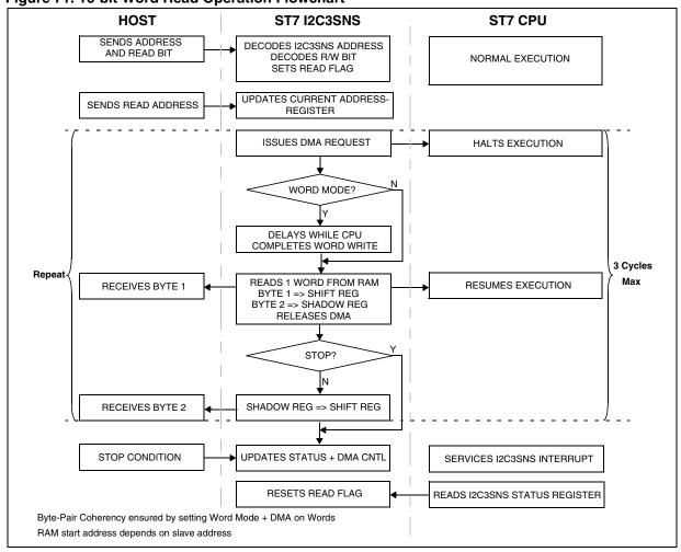
Figure 71. 16-bit Word Read Operation Flowchart
