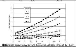
Figure 90. Typical I<sub>DD</sub> in WAIT at f<sub>CPU</sub>= 8MHz
