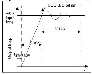
When the PLL is started, after reset or wakeup from Halt mode or AWUFH mode, it outputs the clock after a delay of t<sub>STARTUP</sub>.
