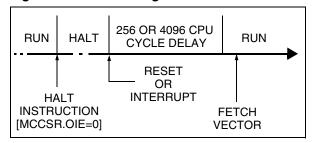
Figure 29. HALT Mode Flow-chart
