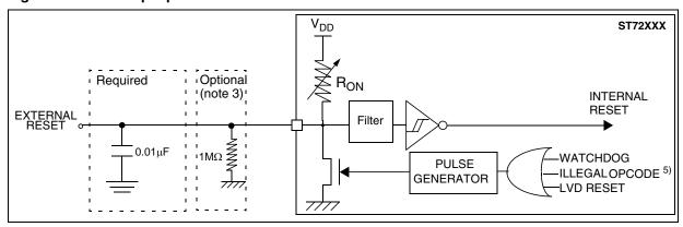
Figure 113. RESET pin protection when LVD is disabled. 1)
