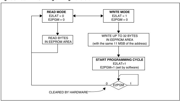
Figure 9. Data E<sup>2</sup>PROM Write Operation
