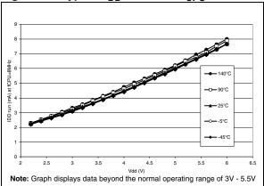
Figure 88. Typical I<sub>DD</sub> in SLOW vs. f<sub>CPU</sub>
