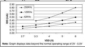
Figure 89. Typical I<sub>DD</sub> in WAIT vs. f<sub>CPU</sub>
