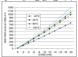
Figure 110. Typical  $V_{DD}$ - $V_{OH}$  at  $V_{DD}$ =5V (std) 1000 900 - -45°C VDD-VOH (mV) at VDD=5 V 800 25°C 700 90°C 600 130°C 500 400 300 200 100
