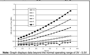
Figure 91. Typical I<sub>DD</sub> in SLOW-WAIT vs. f<sub>CPU</sub>
