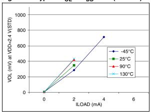
Figure 97. Typical V<sub>OL</sub> at V<sub>DD</sub>=3V (std I/Os)
