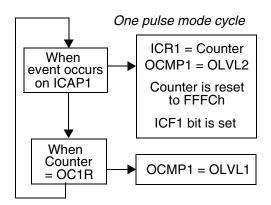
When a valid event occurs on the ICAP1 pin, the counter value is loaded in the ICR1 register. The counter is then initialized to FFFCh, the OLVL2 bit is output on the OCMP1 pin and the ICF1 bit is set.
