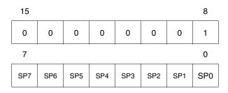
The Stack Pointer is a 16-bit register which is always pointing to the next free location in the stack. It is then decremented after data has been pushed onto the stack and incremented before data is popped from the stack (see Figure 12).
