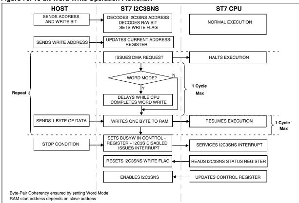
Figure 70. 16-bit Word Write Operation Flowchart
