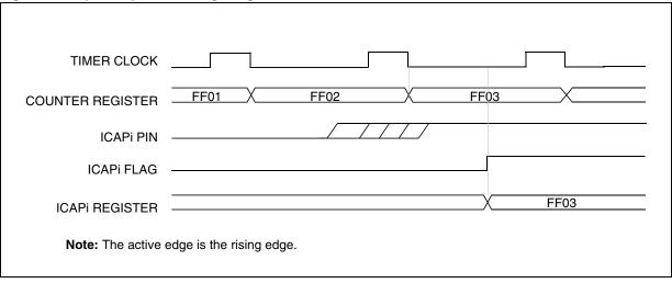
**Note:** The time between an event on the ICAPi pin and the appearance of the corresponding flag is from 2 to 3 CPU clock cycles. This depends on the moment when the ICAP event happens relative to the timer clock.
