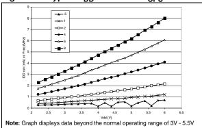
Figure 87. Typical  $I_{DD}$  in RUN at  $f_{CPU} = 8MHz$
