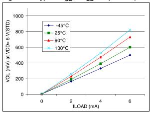
Figure 99. Typical  $V_{OL}$  at  $V_{DD}$ =2.4V (high-sink I/Os)
