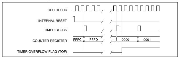
Figure 45. Counter Timing Diagram, internal clock divided by 8
