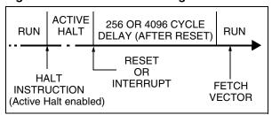
Figure 31. ACTIVE-HALT Mode Flow-chart
