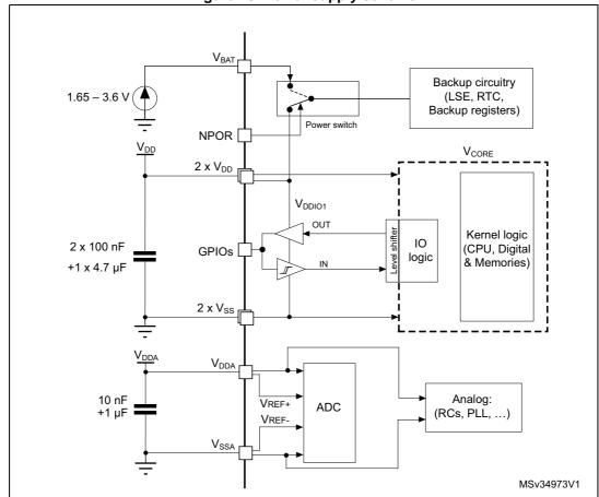
Figure 10. Power supply scheme
