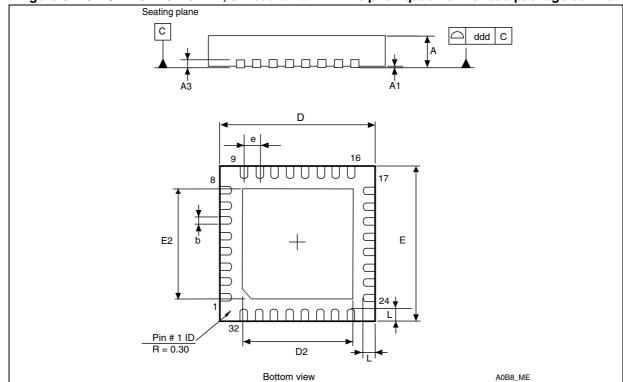
Figure 31. UFQFPN32 - 5 x 5 mm, 32-lead ultra thin fine pitch quad flat no-lead package outline
