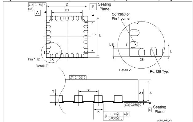
Figure 33. UFQFPN28 - 4 x 4 mm, 28-lead ultra thin fine pitch quad flat no-lead package outline
