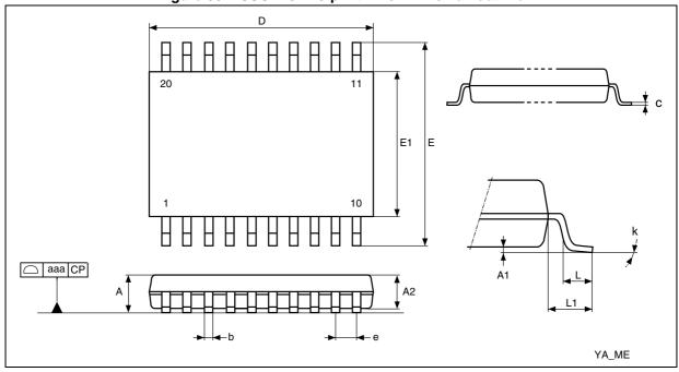
Figure 35. TSSOP20 - 20-pin thin shrink small outline
