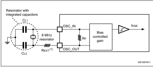
Figure 14. Typical application with an 8 MHz crystal
