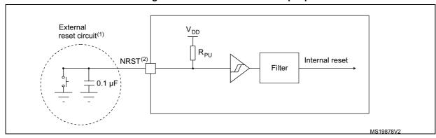
Figure 21. Recommended NRST pin protection
