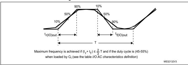
Figure 20. I/O AC characteristics definition
