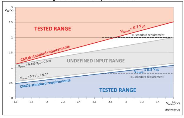
Figure 18. TC and TTa I/O input characteristics
