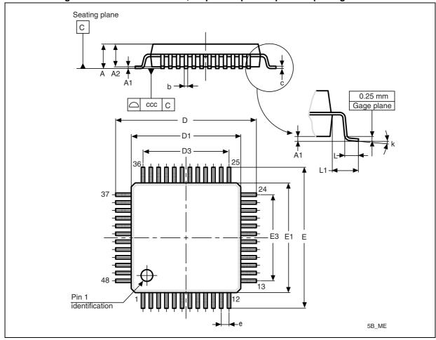
Figure 29. LQFP48 - 7 x 7 mm, 48-pin low-profile quad flat package outline
