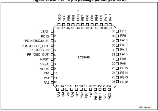
Figure 5. LQFP48 48-pin package pinout (top view)
