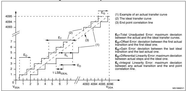
Figure 24. ADC accuracy characteristics
