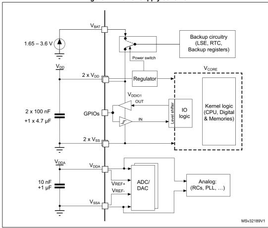
Figure 12. Power supply scheme
