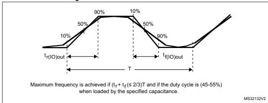
Figure 22. I/O AC characteristics definition
