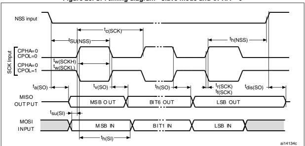
Figure 28. SPI timing diagram - slave mode and CPHA = 0
