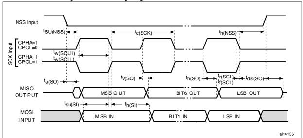
Figure 29. SPI timing diagram - slave mode and CPHA = 1
