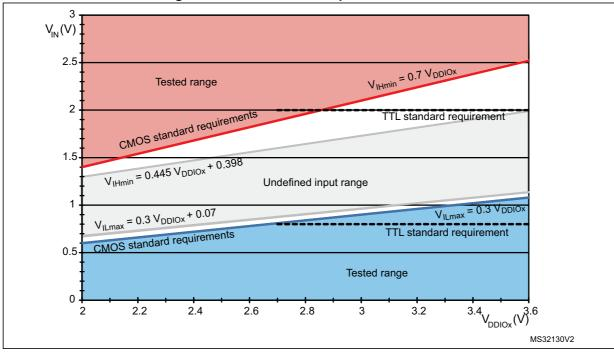
Figure 20. TC and TTa I/O input characteristics
