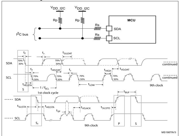
Figure 27. I<sup>2</sup>C bus AC waveforms and measurement circuit
