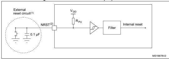
Figure 23. Recommended NRST pin protection
