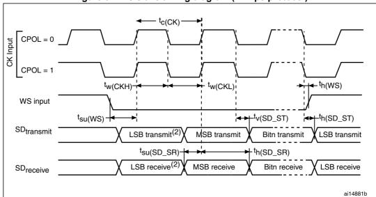
Figure 31. I2S slave timing diagram (Philips protocol)
