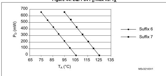
Figure 44. LQFP64 PD max vs. TA
