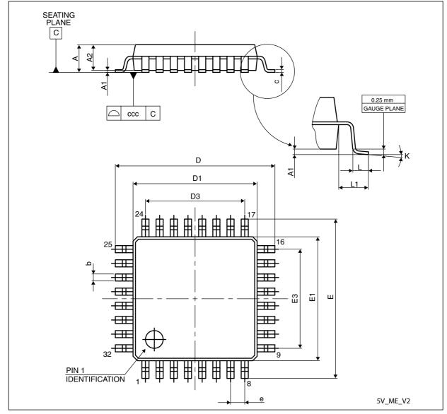
Figure 37. LQFP32 - 7 x 7mm 32-pin low-profile quad flat package outline
