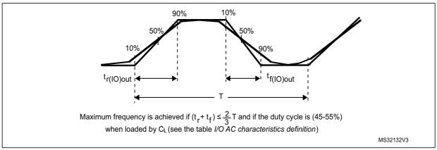
Figure 19. I/O AC characteristics definition
