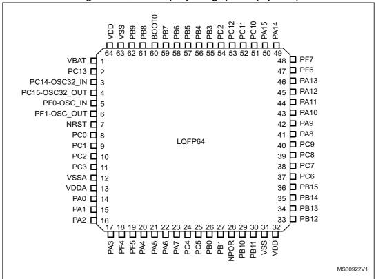
Figure 4. LQFP64 64-pin package pinout (top view)
