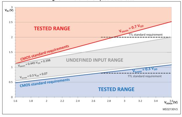
Figure 17. TC and TTa I/O input characteristics
