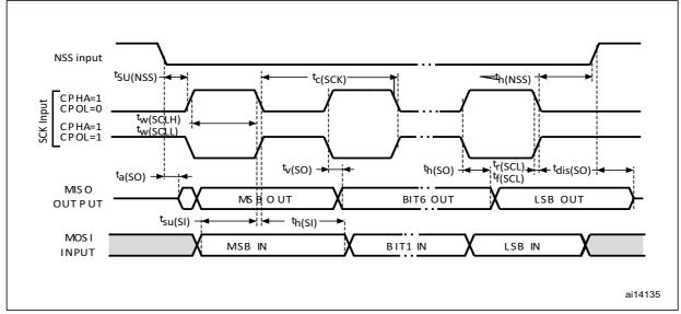
1. Measurement points are done at CMOS levels: 0.3  $V_{DD}$  and 0.7  $V_{DD}$ .
