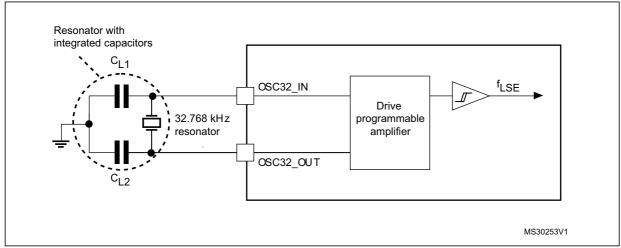
Figure 14. Typical application with a 32.768 kHz crystal
