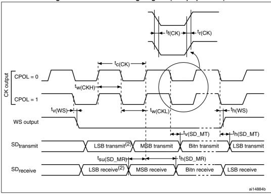
Figure 28. I2S master timing diagram (Philips protocol)
