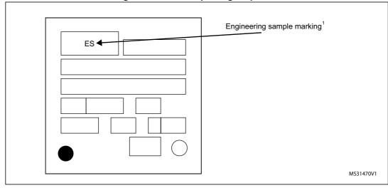
Figure 31. LQFP64 package top view
