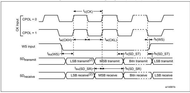
Figure 27. I2S slave timing diagram (Philips protocol)
