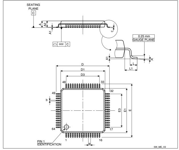
Figure 29. LQFP64 – 10 x 10 mm 64 pin low-profile quad flat package outline
