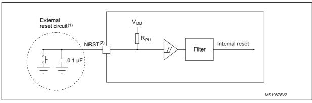
Figure 20. Recommended NRST pin protection
