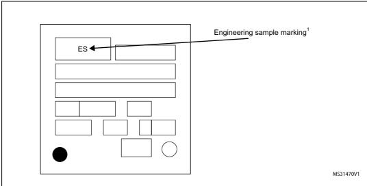
Figure 39. LQFP64 package top view
