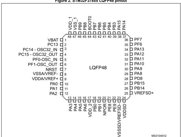
Figure 2. STM32F378xx LQFP48 pinout
