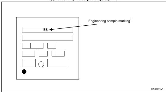
Figure 36. LQFP100 package top view
