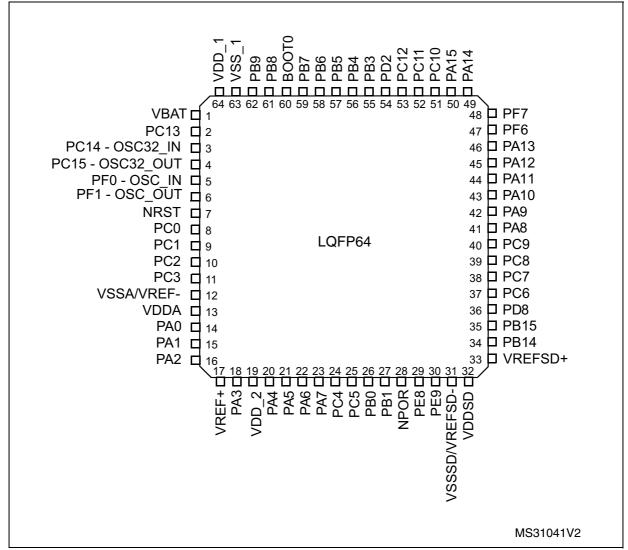
Figure 3. STM32F378xx LQFP64 pinout
