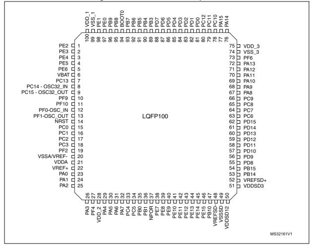
Figure 4. STM32F378xx LQFP100 pinout
