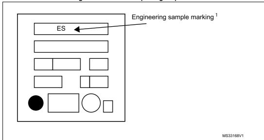
Figure 31. UFBGA100 package top view
