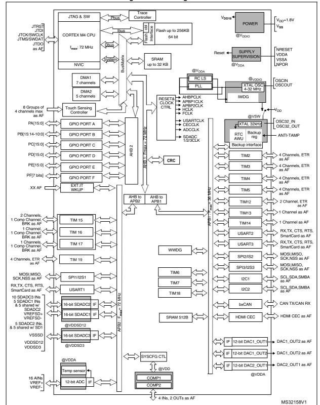
Figure 1. Block diagram
