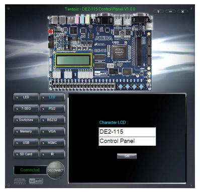
Figure 3-5 Controlling the LCD display
