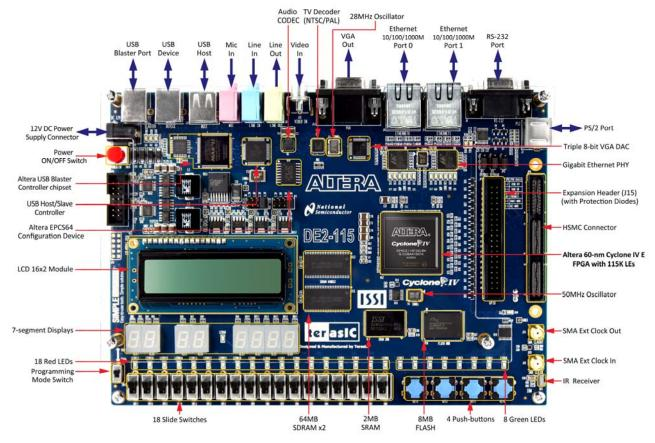
Figure 2-1 The DE2-115 board (top view)
