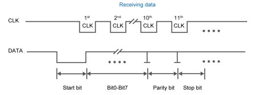
Figure 6-16 Waveforms on two lines while communication taking place
