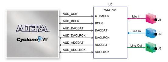
Figure 4-23 Connections between FPGA and Audio CODEC
