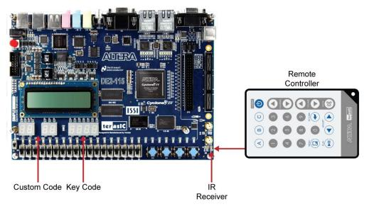
Figure 6-22 The Setup of the IR receiver demonstration
