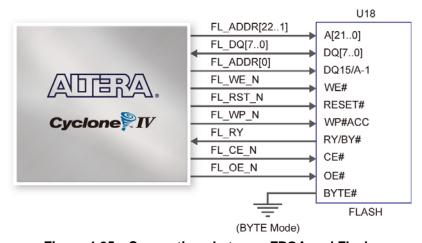
Figure 4-35 Connections between FPGA and Flash
