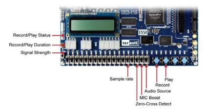
Figure 6-25 Man-Machine Interface of Audio Recorder and Player
