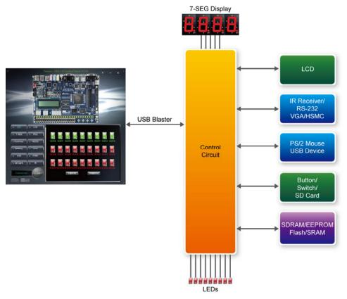
Figure 3-2 The DE2-115 Control Panel concept
