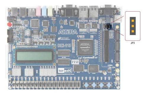
Figure 4-2 The JTAG chain configuration header
