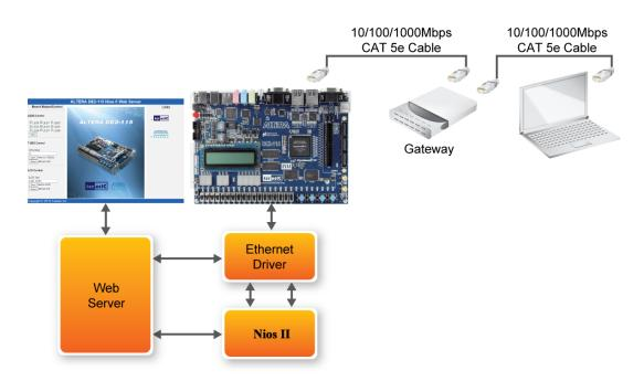
Figure 6-34 System Principle Diagram
