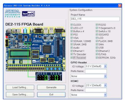
Figure 5-2 The DE2-115 System Builder window
