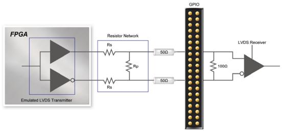
Figure 4-19 Using Emulated LVDS on GPIO
