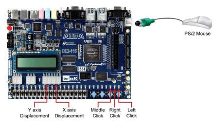
Figure 6-17 The setup of the PS/2 Mouse demonstration
