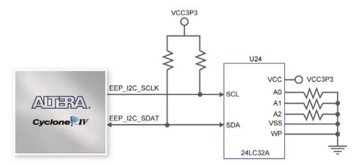
Figure 4-36 Connections between FPGA and EEPROM
