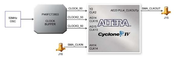
Figure 4-11 Block diagram of the clock distribution
