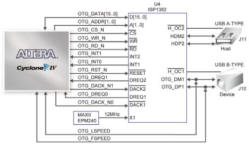
Figure 4-31 Connections between FPGA and USB (ISP1362)
