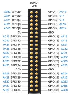
Figure 4-15 GPIO Pin Arrangement
