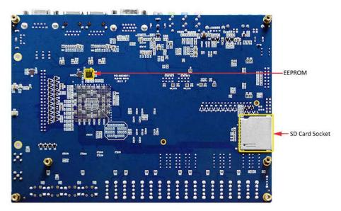
Figure 2-2 The DE2-115 board (bottom view)
