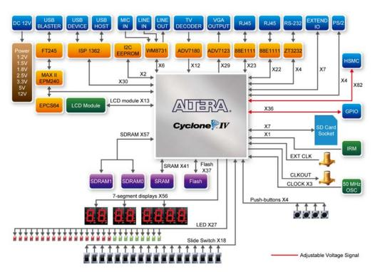
Figure 2-3 Block Diagram of DE2-115
