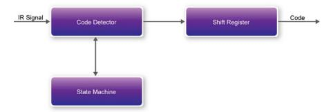
Figure 6-20 The IR Receiver controller
