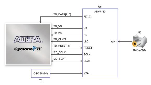
Figure 4-29 Connections between FPGA and TV Decoder
