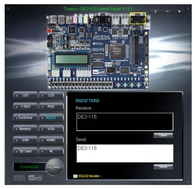
Figure 3-11 RS-232 Serial Communication
