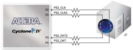
Figure 4-25 Connection between FPGA and PS/2
