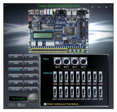
Figure 3-6 Monitoring switches and buttons
