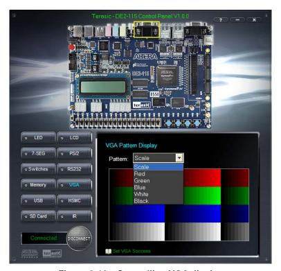
Figure 3-12 Controlling VGA display
