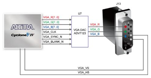
Figure 4-21 Connections between FPGA and VGA
