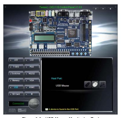
Figure 3-8 USB Mouse Monitoring Tool
