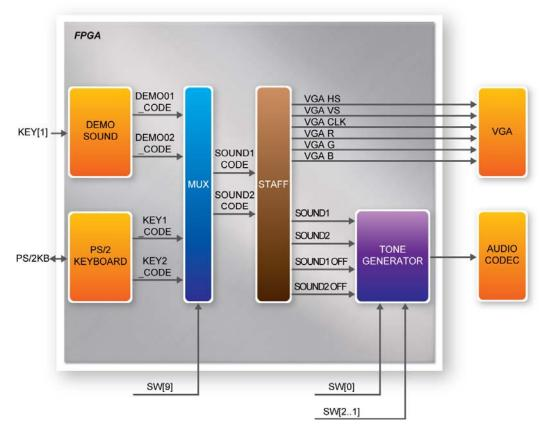
Figure 6-23 Block diagram of the Music Synthesizer design
