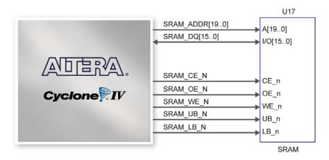
Figure 4-33 Connections between FPGA and SRAM
