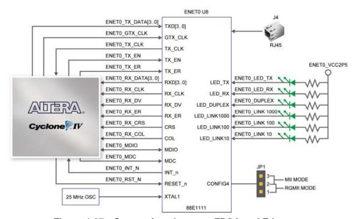
Figure 4-27 Connections between FPGA and Ethernet
