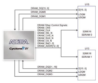
Figure 4-34 Connections between FPGA and SDRAM
