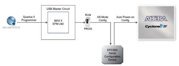
Figure 4-5 The AS configuration scheme
