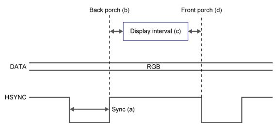
Figure 4-22 VGA horizontal timing specification
