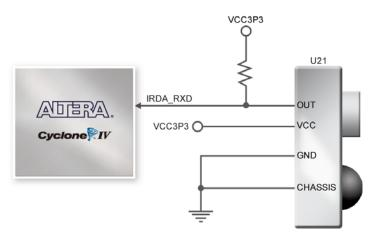
Figure 4-32 Connection between FPGA and IR
