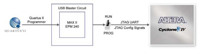
Figure 4-3 The JTAG configuration scheme
