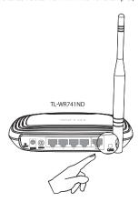
Launch the configuration utility and click WPS in the tools section. Select Push the button on my access point or wireless router and then click Connect.
