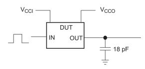
DATA RATE, SKEW, PROPAGATION DELAY, OUTPUT RISE AND FALL TIME MEASUREMENT
