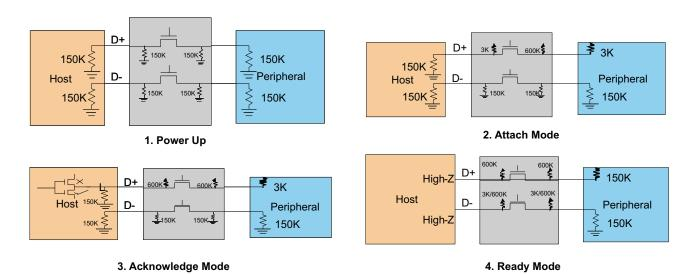
Figure 1. Block Diagram Showing Different Modes in the TXS0202
