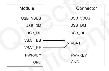
Figure 26: Test Points of Firmware Upgrade
