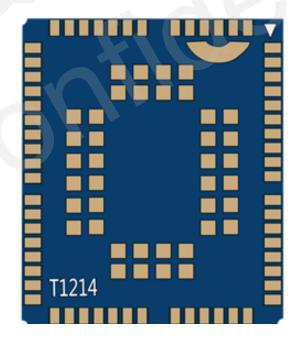
Figure 40: Bottom View of the Module
