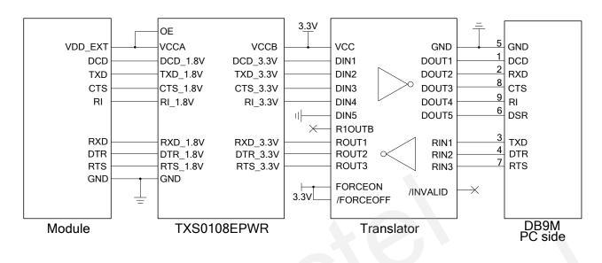
Figure 22: RS232 Level Match Circuit
