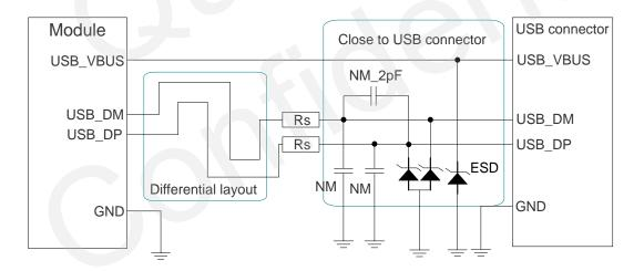
Figure 25: Reference Circuit of USB Application
