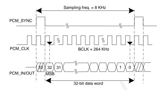
Figure 27: PCM Master Mode Timing
