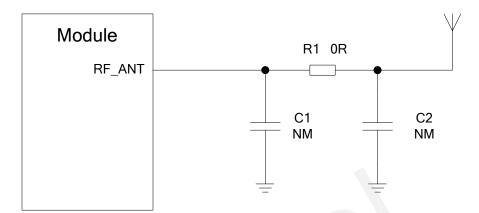
Figure 31: Reference Circuit of Antenna Interface
