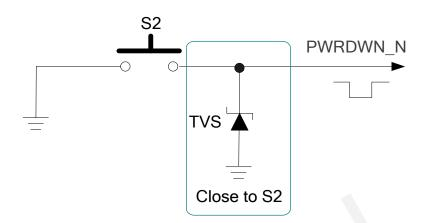
Figure 14: Turn off the Module Using Keystroke
