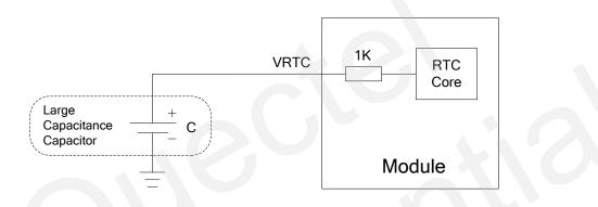
Figure 19: RTC Supply from Capacitor
