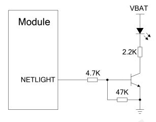
Figure 29: Reference Circuit of the NETLIGHT
