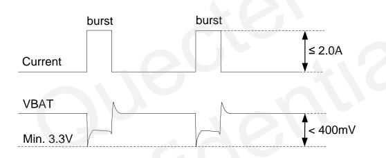
Figure 6: Voltage Drop during Transmitting Burst
