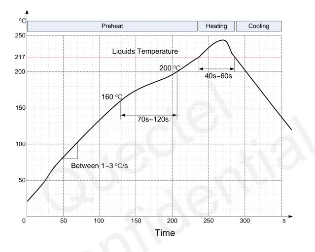
Figure 41: Reflow Soldering Profile
