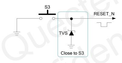
Figure 17: Reference Circuit of RESET\_N by Using Button
