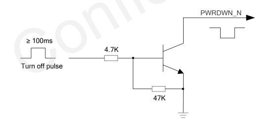
Figure 13: Turn off the Module Using Driving Circuit
