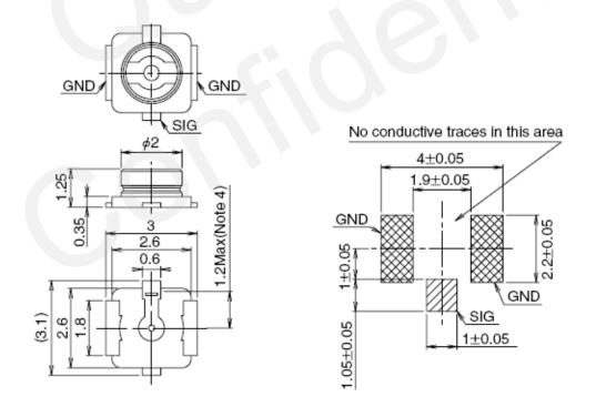
Figure 32: Dimensions of the UF.L-R-SMT Connector (Unit: mm)
