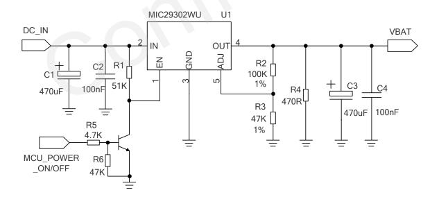
Figure 8: Reference Circuit of Power Supply
