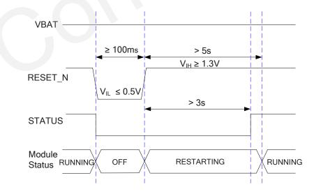
Figure 18: Timing of Resetting Module
