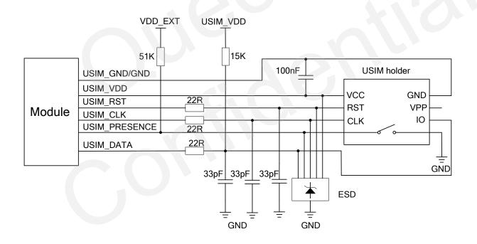
Figure 23: Reference Circuit of the 8-Pin USIM Card
