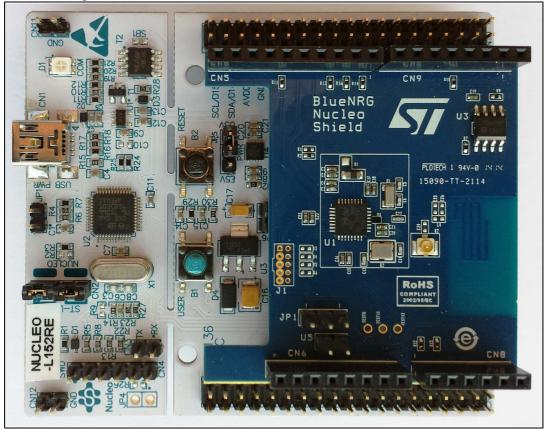
Figure 2. X-NUCLEO-IDB04A1 connected to STM32 Nucleo board
