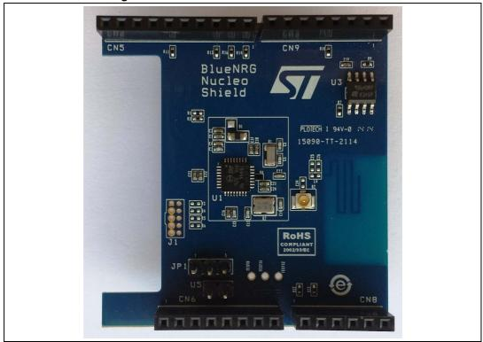
Figure 1. X-NUCLEO-IDB04A1 evaluation board
