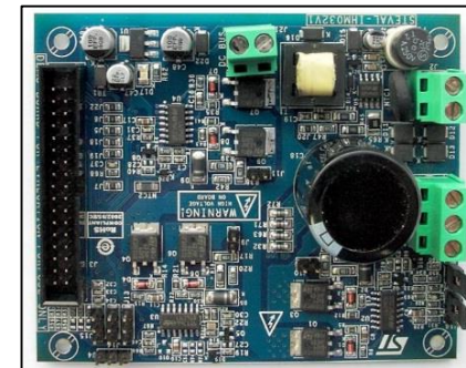
Motor Control Power block
